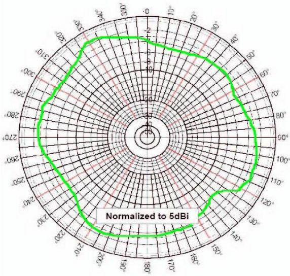
Azimuthal Pattern (X, Y or E-Plane)
