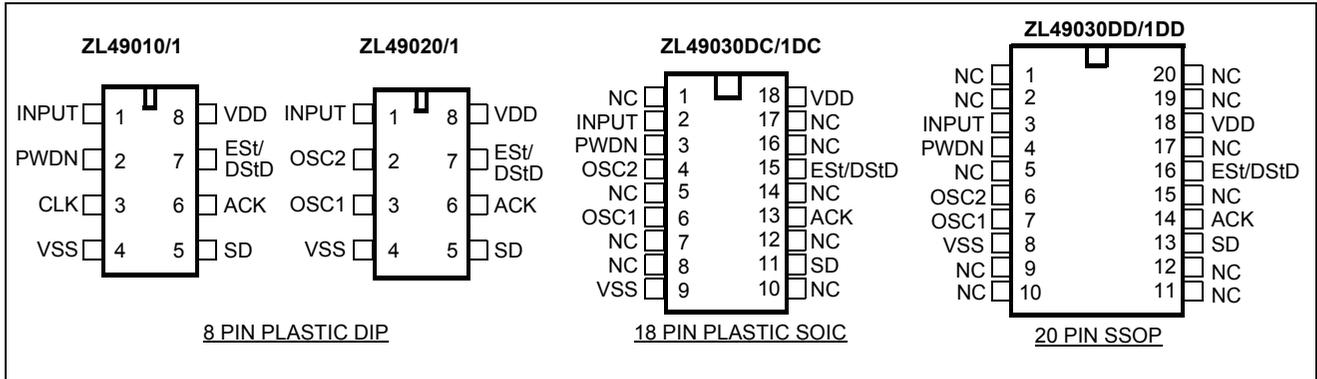
Figure 2 - Pin Connections
