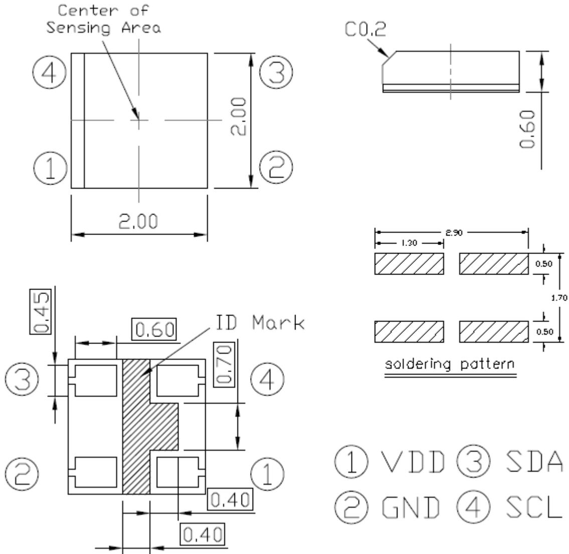
Note: Tolerances unless mentioned  $\pm 0.2$ mm. Unit = mm
