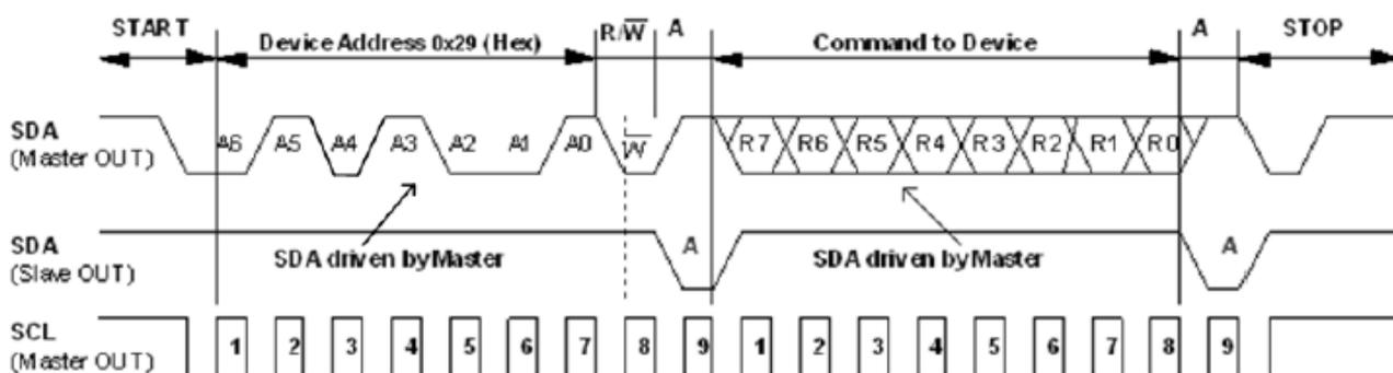
Figure 14. I<sup>2</sup>C Timing Diagram for Send Byte Format
