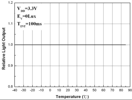
**Fig 10. Light Output vs. Temperature**
