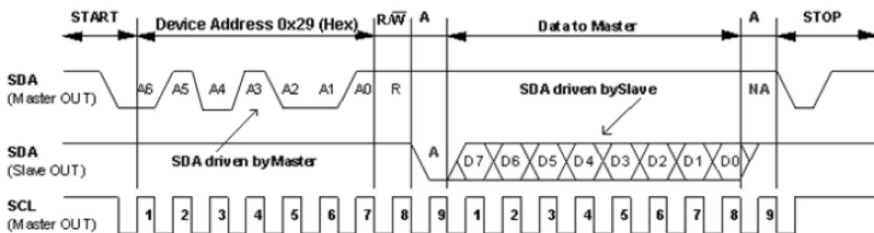
Figure 15. I<sup>2</sup>C Timing Diagram for Receive Byte Format
