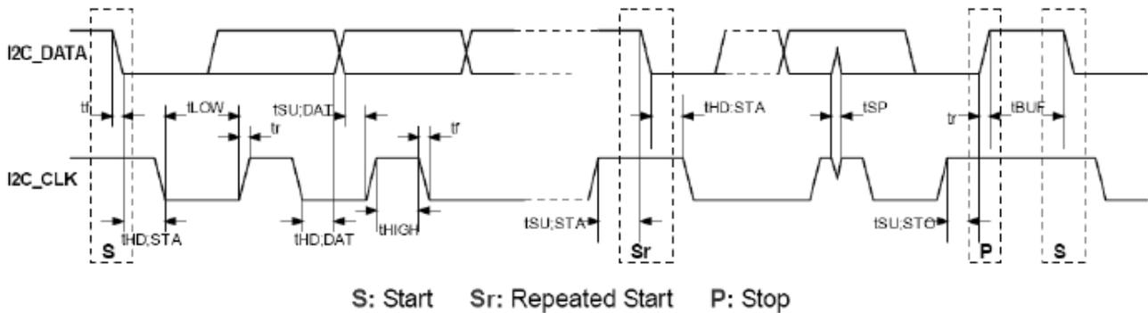
Figure 2. I<sup>2</sup>C Timing Diagram
