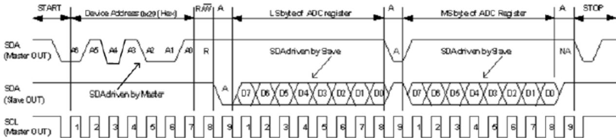
Figure 16. I<sup>2</sup>C Timing Diagram for Receive Word Format
