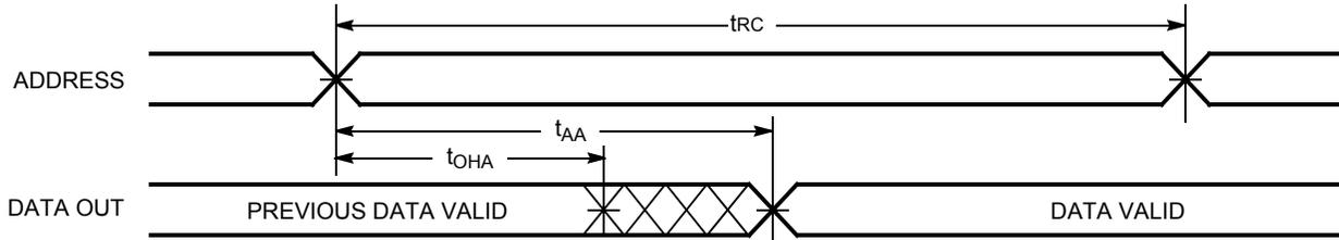
Figure 5. Read Cycle No. 2 ( $\overline{OE}$  Controlled) [15, 16]
