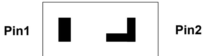
*Note: Product marking may be rotated by multiples of 90° for assembly plant differentiation. In no case should this product marking be used to orient the component for its placement on a PCB. Only pin 1 mark is to be used for this purpose.*
