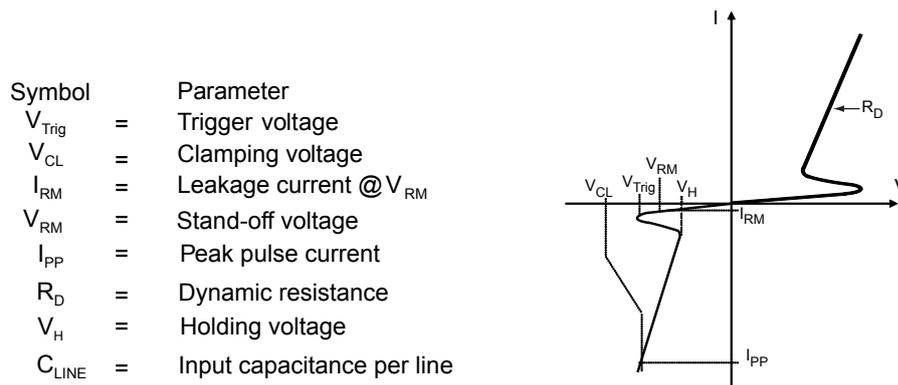
**Table 2. Electrical characteristics ( $T_{amb} = 25\text{ °C}$ )**
