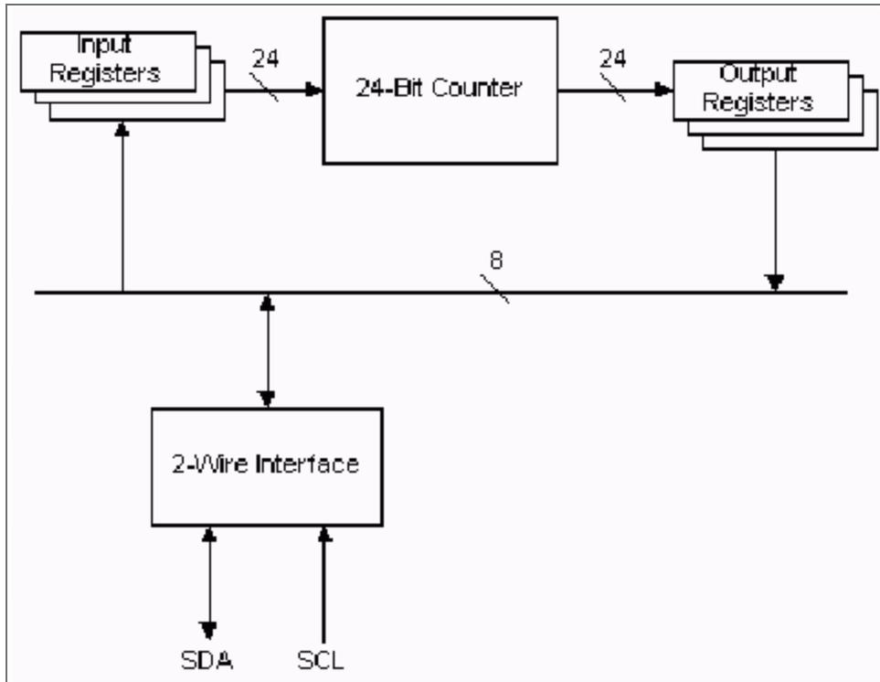
Figure 1. Watchdog/Alarm counter configuration.
