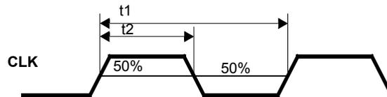
**Figure 1. Duty Cycle Definition; DC =  $t_2/t_1$**
