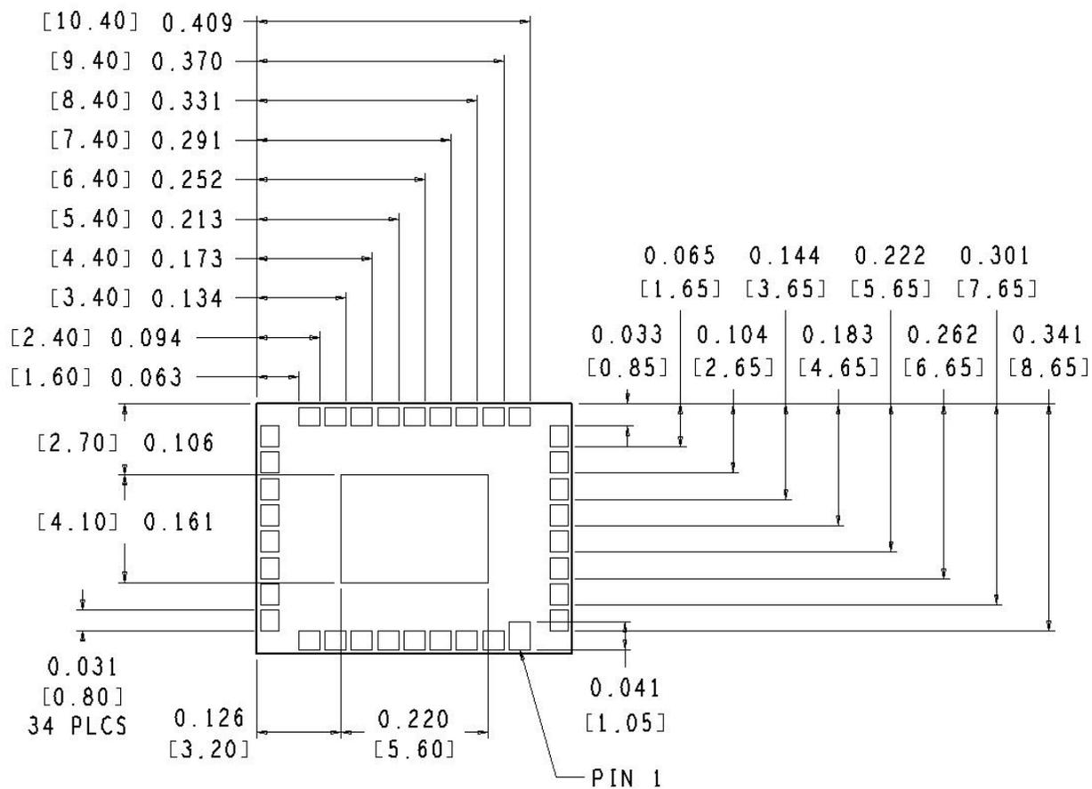
The nominal size of the part is 10x13mm with a height of 1.7mm
