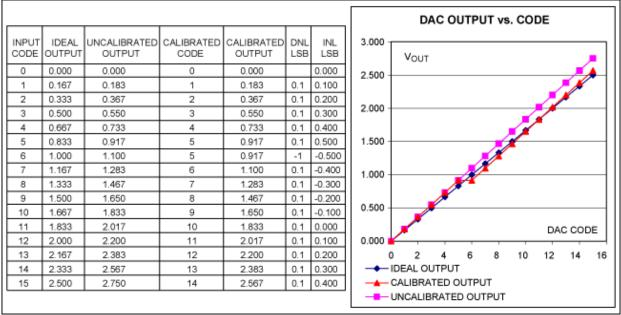
Figure 3. A digitally calibrated DAC system.
