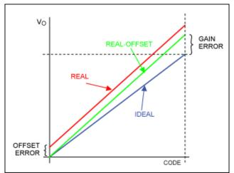
Figure 1. Gain and offset errors.
