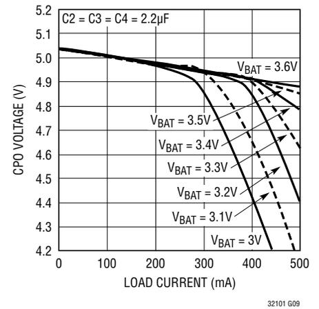
**TYPICAL PERFORMANCE CHARACTERISTICS**  $T_A = 25^\circ\text{C}$ , unless otherwise stated.
