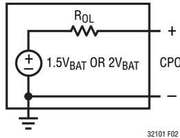
**Figure 2. Charge Pump Thevenin Equivalent Open-Loop Circuit**
