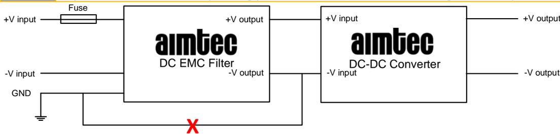
**Note:** Connections marked with **X** interfere with this filter modules performance and should therefore not be used
