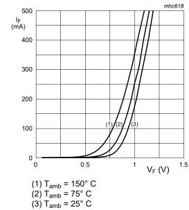
Forward current as a function of forward Fig. 3. voltage; typical values
