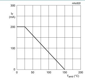
Forward current as a function of ambient temperature; derating curve
