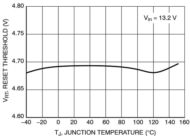
Figure 22. Reset Threshold vs Temperature (5 V option)
