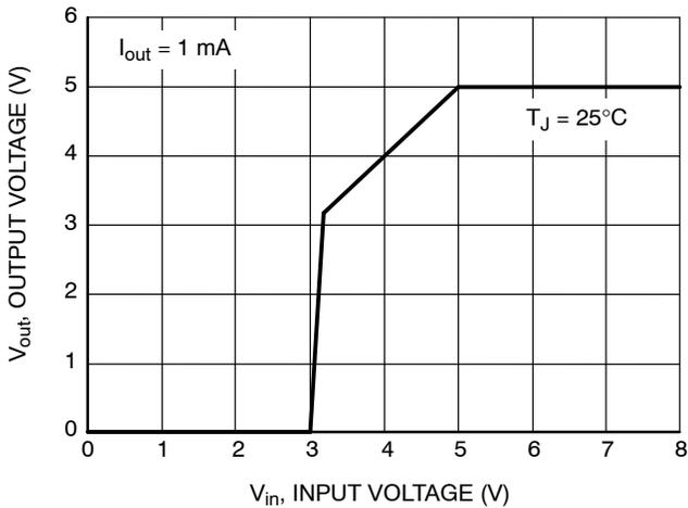
Figure 8. Output Voltage vs Input Voltage (5 V option)
