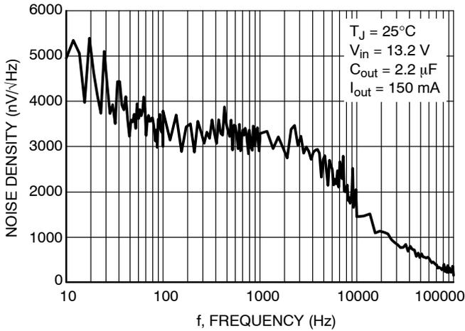
Figure 18. Noise vs. Frequency (5 V option)
