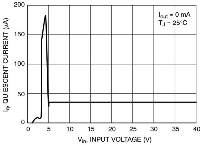
Figure 5. Quiescent Current vs Input Voltage (5 V option)
