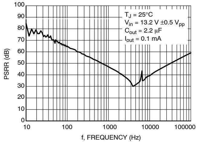
Figure 17. PSRR vs. Frequency (5 V option)
