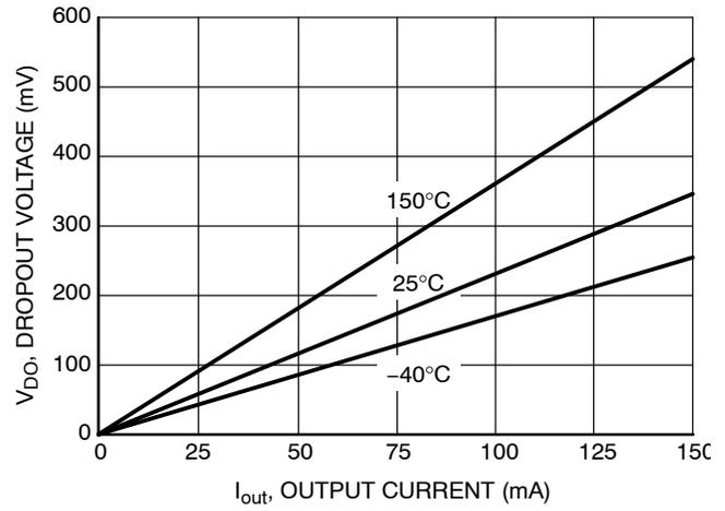
Figure 9. Dropout Voltage vs Output Current (5 V option)
