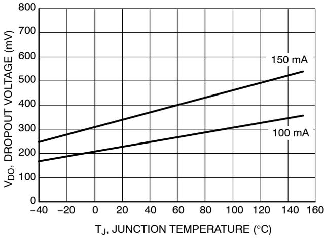
Figure 10. Dropout vs Temperature (5 V option)
