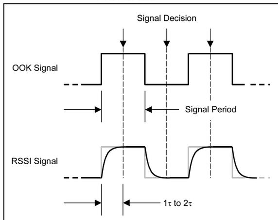
If the bit decision occurs near the end of the signal period, then the time constant should be set at less than or equal to the signal period. Figure 3-11 illustrates this method.
