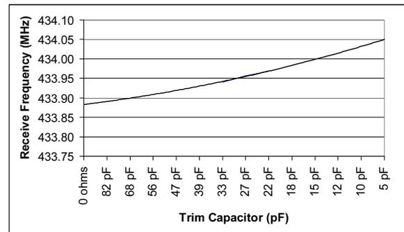
Note that a 0  $\Omega$  resistor, in the lower left of the graph, represents an infinite capacitance. This will be the lowest frequency obtainable for the crystal and PCB combination.
