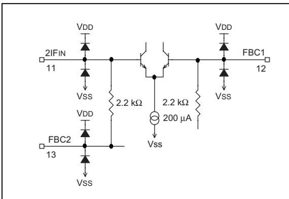
**FIGURE 2-8: BLOCK DIAGRAM OF IF LIMITING AMPLIFIER OUTPUT PIN**
