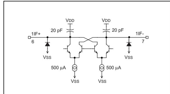
**FIGURE 2-6: BLOCK DIAGRAM OF IF PREAMP PIN**
