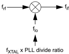
**Step 2:** Calculate crystal frequencies for high- and low-side injection:
