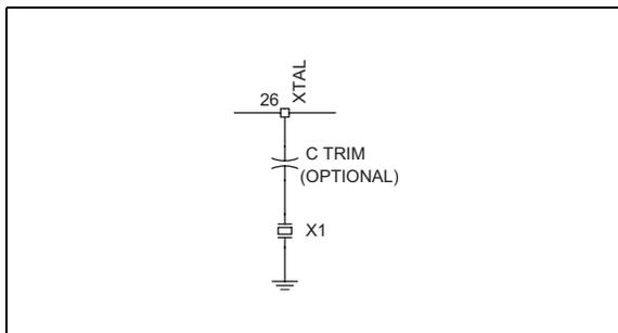
The crystal load capacitance should be specified to include the internal load capacitance of the XTAL pin of 15 pF plus PCB stray capacitance (approximately 2 to 3 pF). A trim capacitor can be used to trim the crystal on frequency within the limitations of the crystal's trim sensitivity and pullability. Figure 3-2 illustrates the
