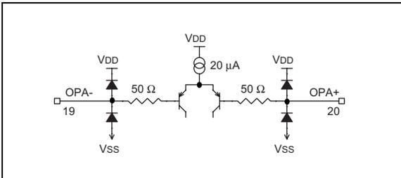
**FIGURE 2-13: BLOCK DIAGRAM OF OP AMP OUTPUT PIN**
