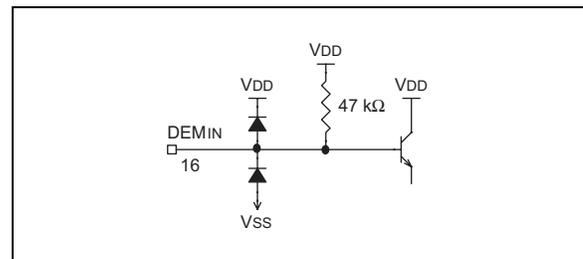
**FIGURE 2-11: BLOCK DIAGRAM OF DEMODULATOR OUTPUT PINS**
