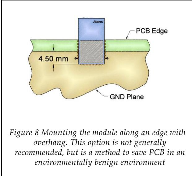
Figure 8 Mounting the module along an edge with overhang. This option is not generally recommended, but is a method to save PCB in an environmentally benign environment
