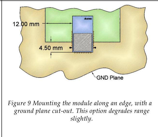
Figure 9 Mounting the module along an edge, with a ground plane cut-out. This option degrades range slightly.
