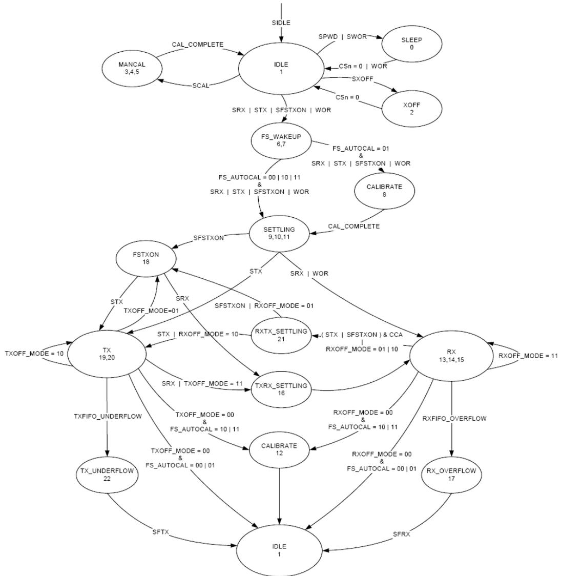
Figure 4 Transceiver state diagram
