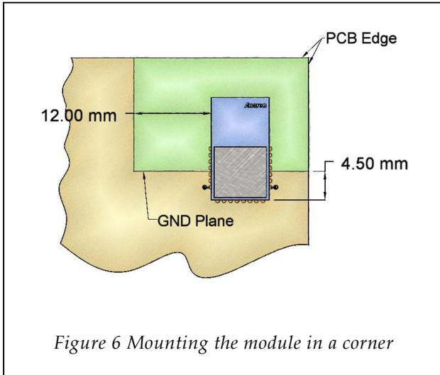
Figure 6 Mounting the module in a corner
