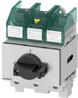
SENTRON, Molded case switch 3LD5 UL, Main switch, 3-pole, certified according to UL489 UL60947-4-1 and IEC60947-3, UL: 60A, SCCR 50kA at 480VAC, Operating power at 480VAC 3-phase: 40hp, IEC: 63A, Operating power at AC-23A at 400V: 30kW, floor mounting with direct handle, black, incl. terminal covers for the infeed side
