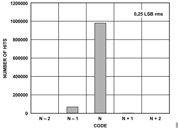
Figure 42. Input-Referred Noise Histogram,  $f_{\text{SAMPLE}} = 125 \text{ MSPS}$
