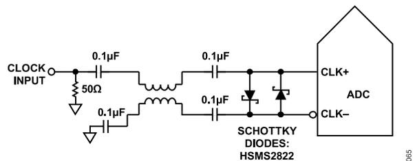
Figure 62. Balun-Coupled Differential Clock (Up to 1 GHz)
