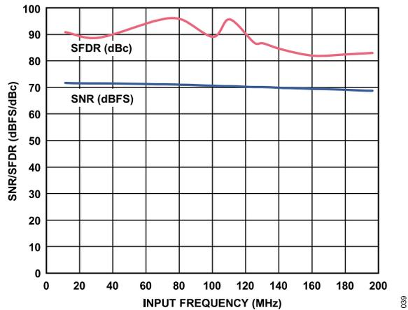
Figure 18. SNR/SFDR vs.  $f_{IN}$ ,  $f_{SAMPLE} = 80$  MSPS
