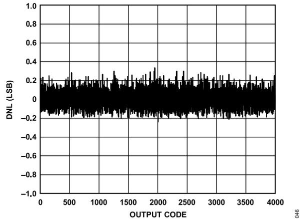
Figure 41. DNL,  $f_{IN} = 9.7$  MHz,  $f_{SAMPLE} = 125$  MSPS
