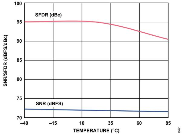
Figure 19. SNR/SFDR vs. Temperature,  $f_{IN} = 10.3$  MHz,  $f_{SAMPLE} = 80$  MSPS
