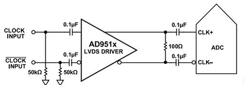
Figure 65. Differential LVDS Sample Clock (Up to 1 GHz)
