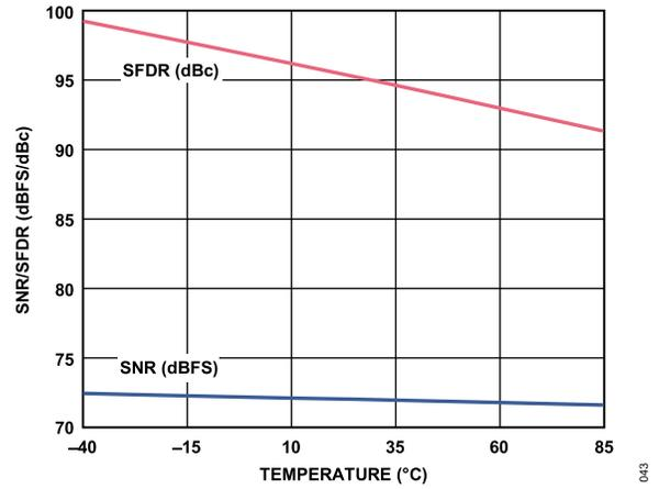
Figure 29. SNR/SFDR vs. Temperature,  $f_{IN} = 10.3$  MHz,  $f_{SAMPLE} = 105$  MSPS
