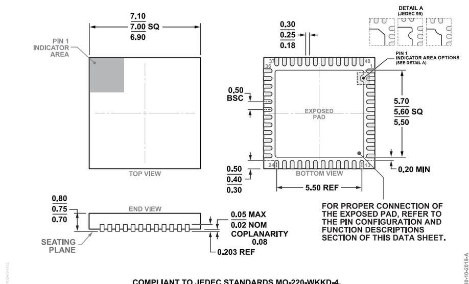
**Figure 78. 48-Lead Lead Frame Chip Scale Package [LFCSP]
