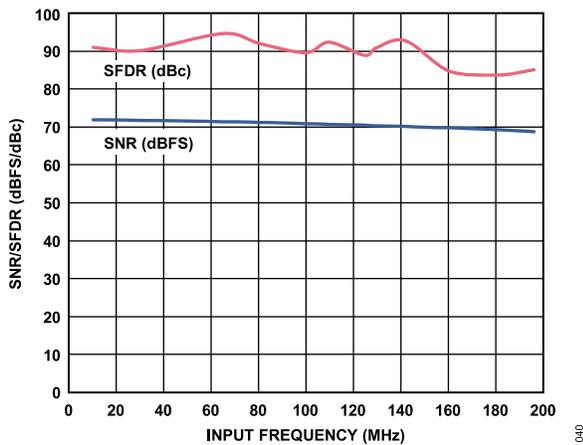
Figure 28. SNR/SFDR vs.  $f_{IN}$ ,  $f_{SAMPLE} = 105$  MSPS
