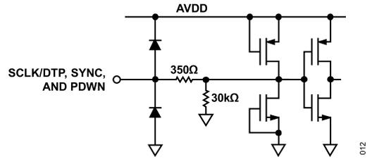
Figure 50. Equivalent SCLK/DTP, SYNC, and PDWN Input Circuit
