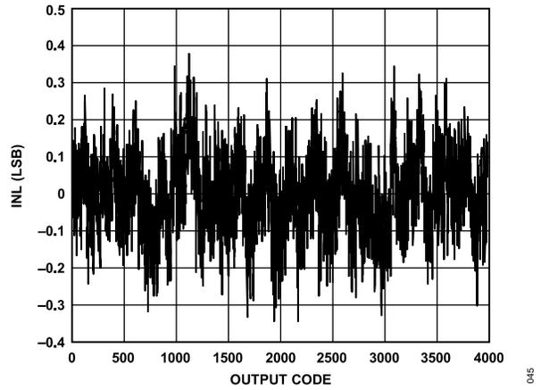
Figure 40. INL,  $f_{IN} = 9.7$  MHz,  $f_{SAMPLE} = 125$  MSPS
