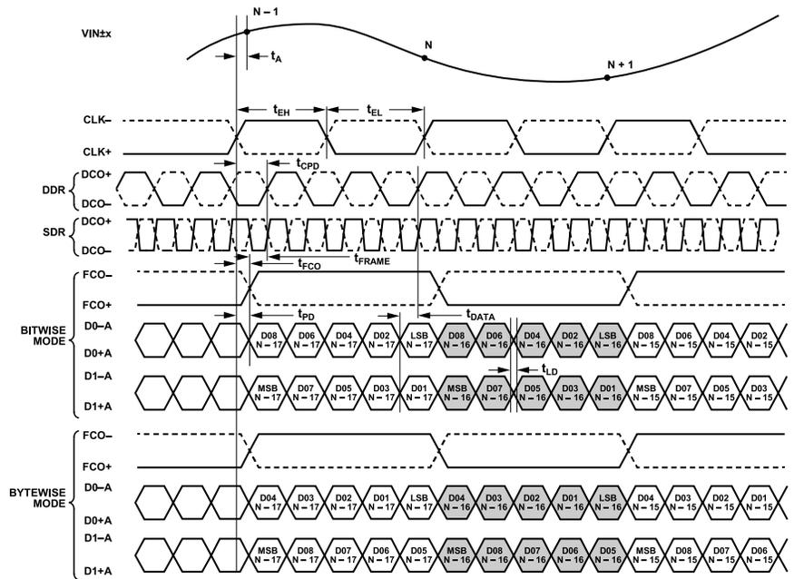
Figure 5. 10-Bit DDR/SDR, Two-Lane, 2x Frame Mode
