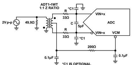
Figure 58. Differential Transformer-Coupled Configuration for Baseband Applications
