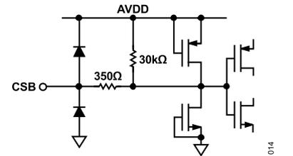
Figure 52. Equivalent CSB Input Circuit
