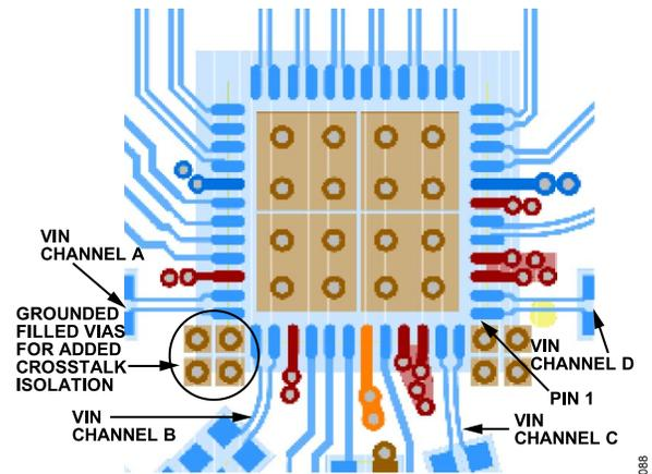
Figure 77. Layout Technique to Maximize Crosstalk Performance
