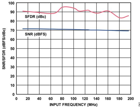
Figure 38. SNR/SFDR vs.  $f_{IN}$ ,  $f_{SAMPLE} = 125$  MSPS
