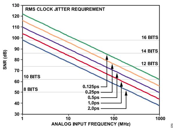
Figure 67. Ideal SNR vs. Input Frequency and Jitter
