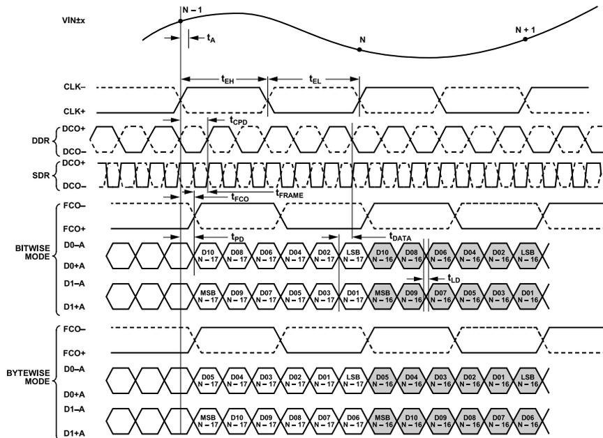
Figure 2. 12-Bit DDR/SDR, Two-Lane, 1x Frame Mode (Default)
