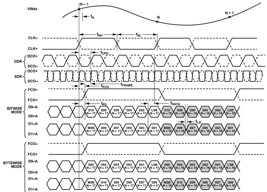
Figure 4. 12-Bit DDR/SDR, Two-Lane, 2x Frame Mode
