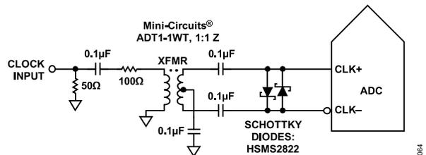
Figure 61. Transformer-Coupled Differential Clock (Up to 200 MHz)
