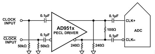
Figure 64. Differential PECL Sample Clock (Up to 1 GHz)
