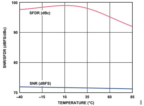
Figure 39. SNR/SFDR vs. Temperature,  $f_{IN} = 10.3$  MHz,  $f_{SAMPLE} = 125$  MSPS
