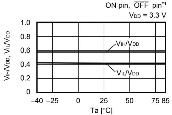
**5. Input threshold voltage (When comparator input is selected)**
