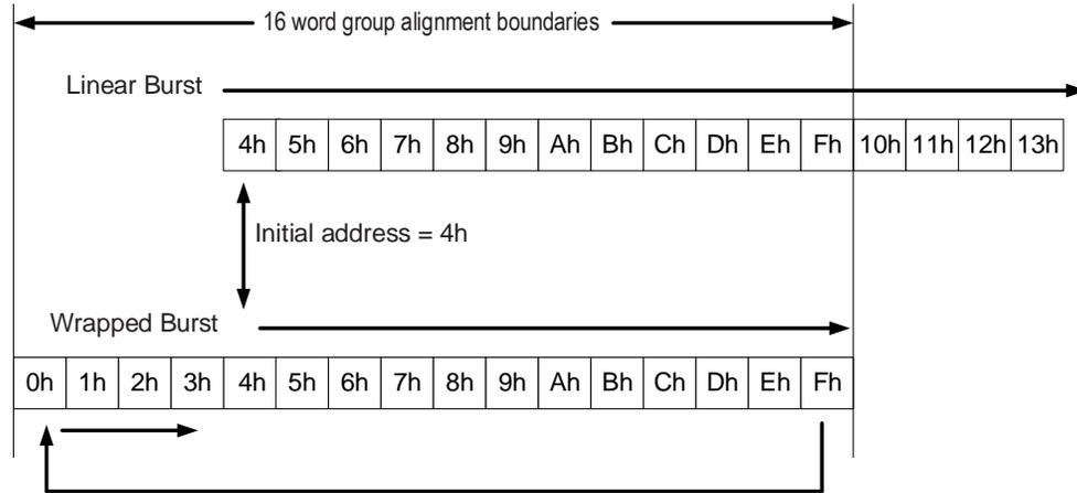
**Figure 4 - Linear Versus Wrapped Burst Sequence**
