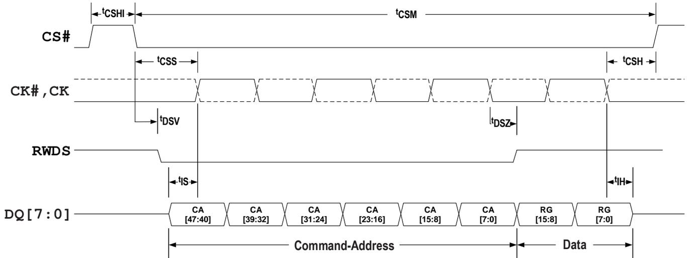
Figure 32 - Write Operation without Initial Latency (Register Write)
