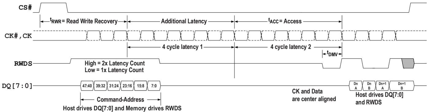
Figure 31 - Write Timing Diagram — With Additional Latency
