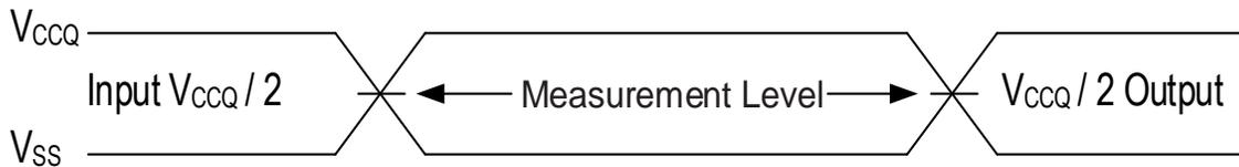
**Figure 25 - Input Waveforms and Measurement Levels**
