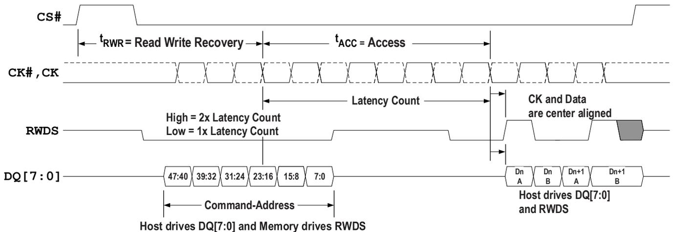
Figure 11 - Write Transaction without Additional Initial Latency
