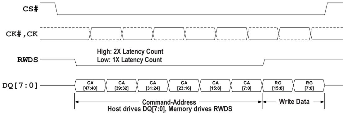
**Figure 12 - Write Operation without Initial Latency**
