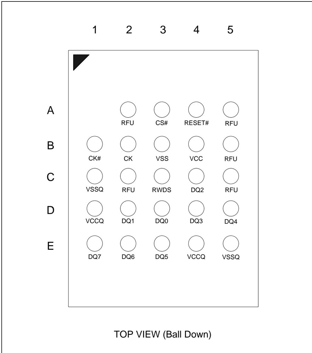
24 Balls TFBGA, 5x5-1 Ball Footprint, Top View
