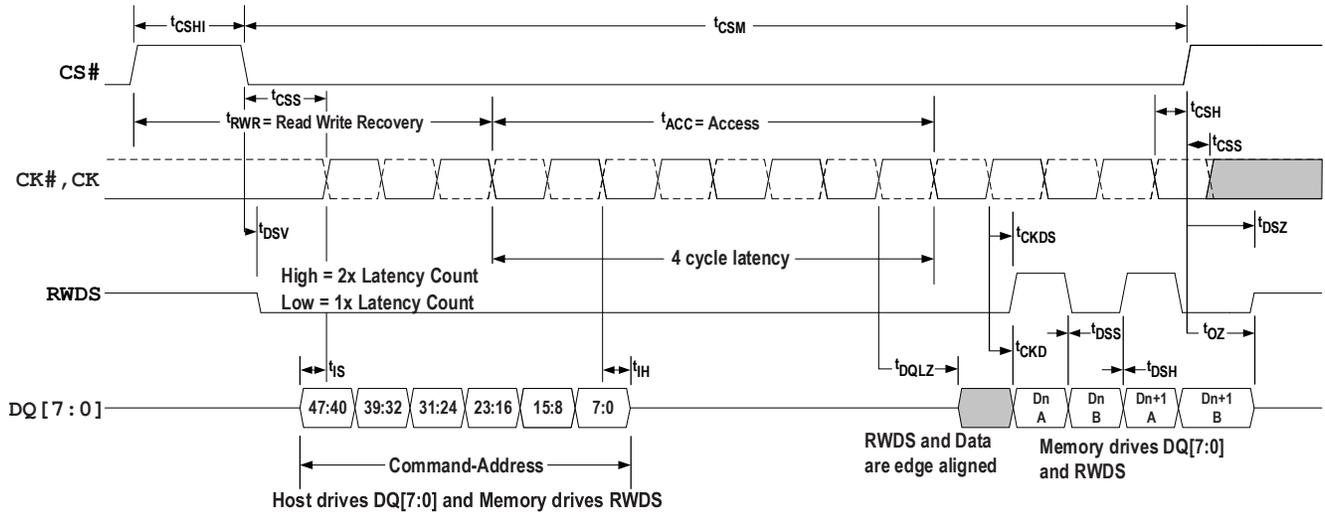
Figure 27 - Read Timing Diagram — No Additional Latency Required
