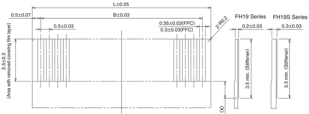
Note1: Polyamide and a thermally hardened adhesive is recommended as the materials for the stiffener.
