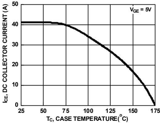
Figure 9. DC Collector Current vs. Case Temperature
