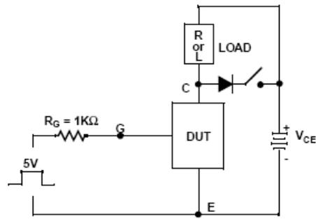
Figure 18.  $t_{ON}$  and  $t_{OFF}$  Switching Test Circuit
