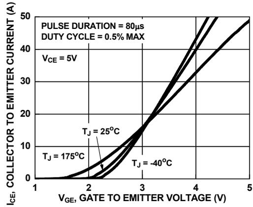
Figure 8. Transfer Characteristics
