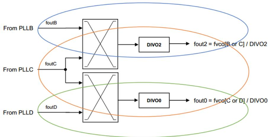
Figure 17 Au5312 & Au5322 Output Clock Distribution
