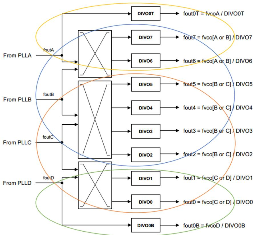
Figure 15 Au5315 & Au5325 Output Clock Distribution
