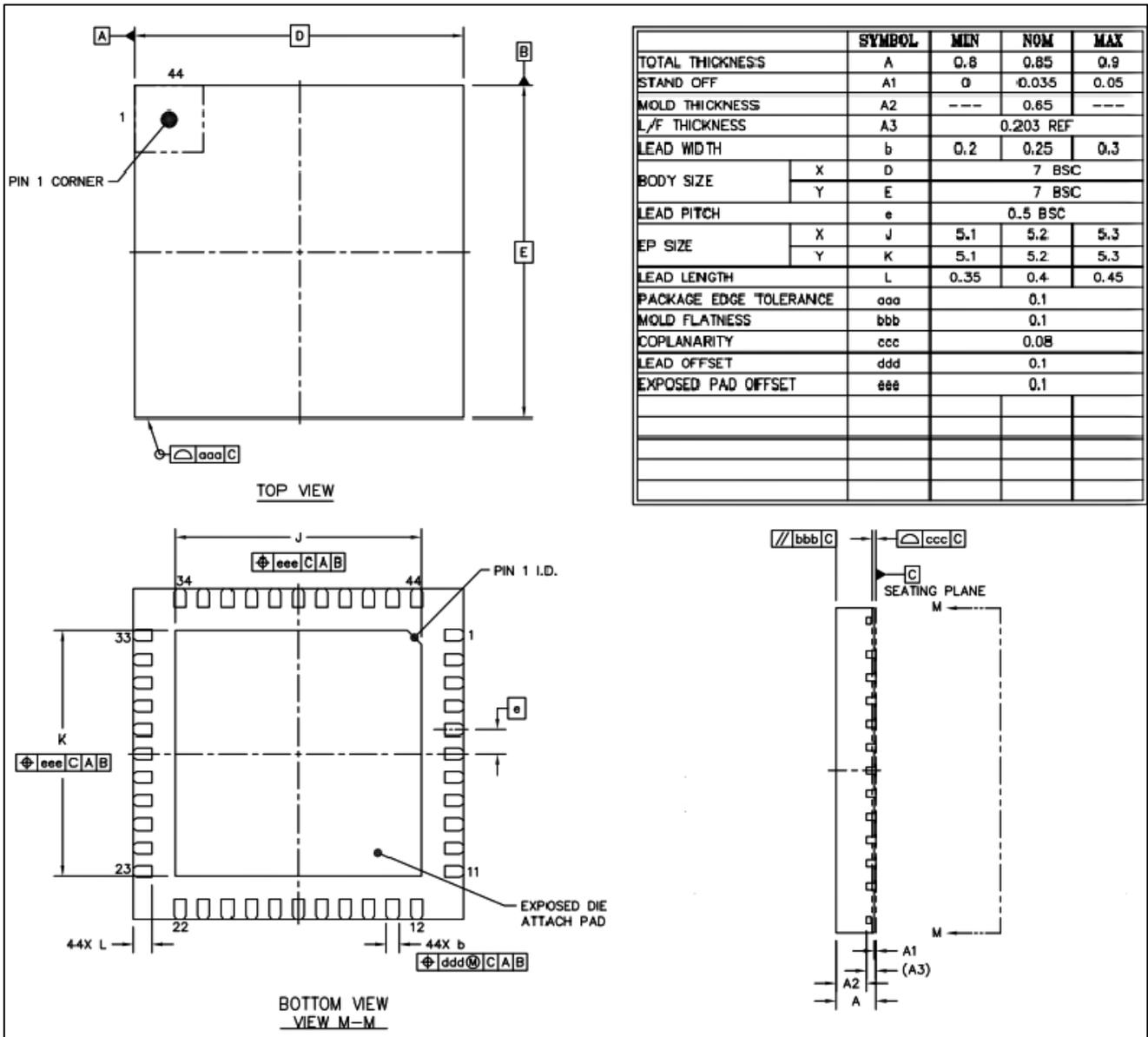
Figure 25 Au53x4 and Au53x2: 44-QFN Package Dimensions
