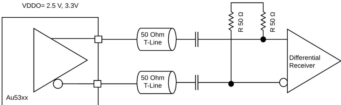
AC Coupled Receiver side termination Option1: Use LVDS Standard for the Au53xx Output Driver
