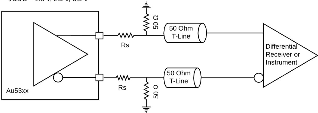
**Figure 34 HCSL DC Coupled Termination. Source Terminated 50 Ohm**
