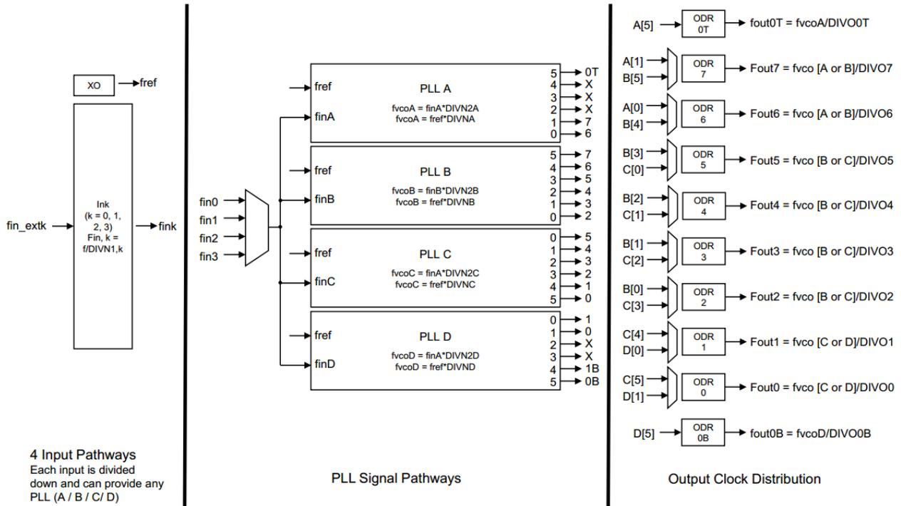
Figure 10 Au5315 & Au5325 Overall Hierarchy of Clocks
