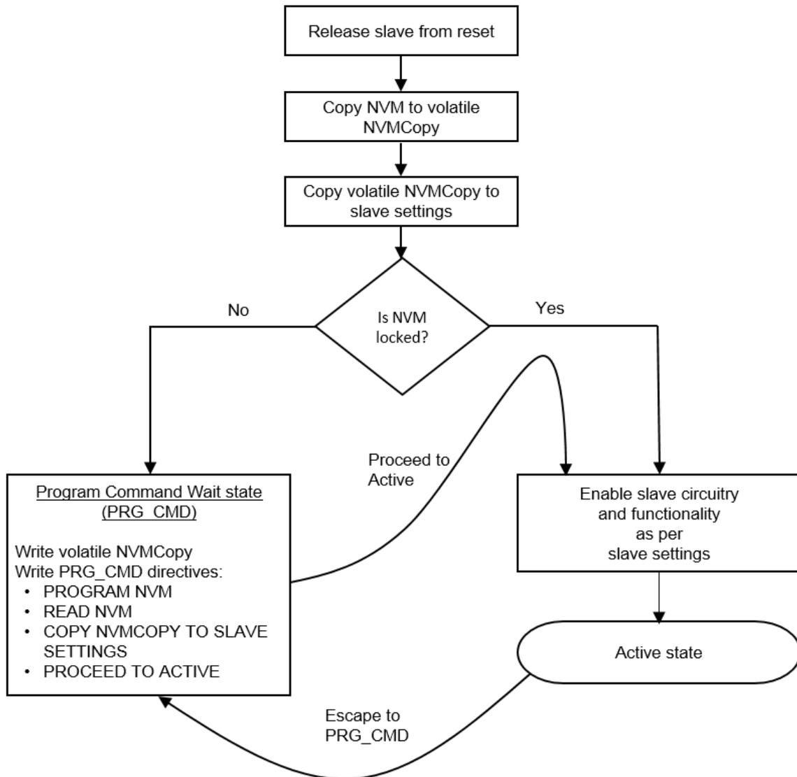
Figure 21 Slave Wake-up Finite State Machine
