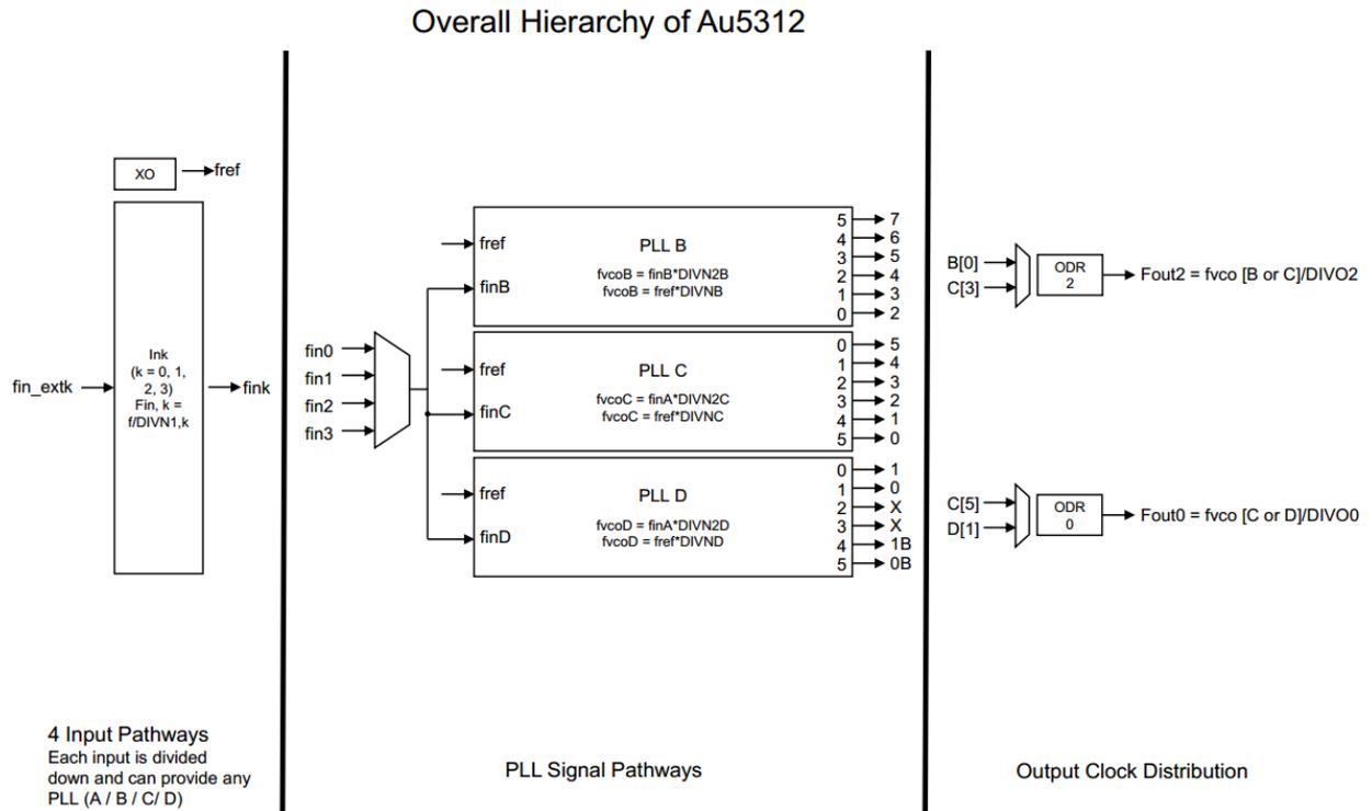
**Figure 12 Au5312 & Au5322 Overall Hierarchy of Clocks**
