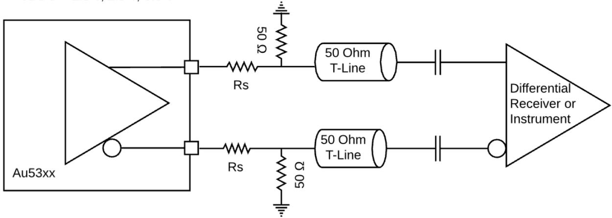
**Figure 33 HCSL AC Coupled Termination. Source Terminated 50 Ohm**
