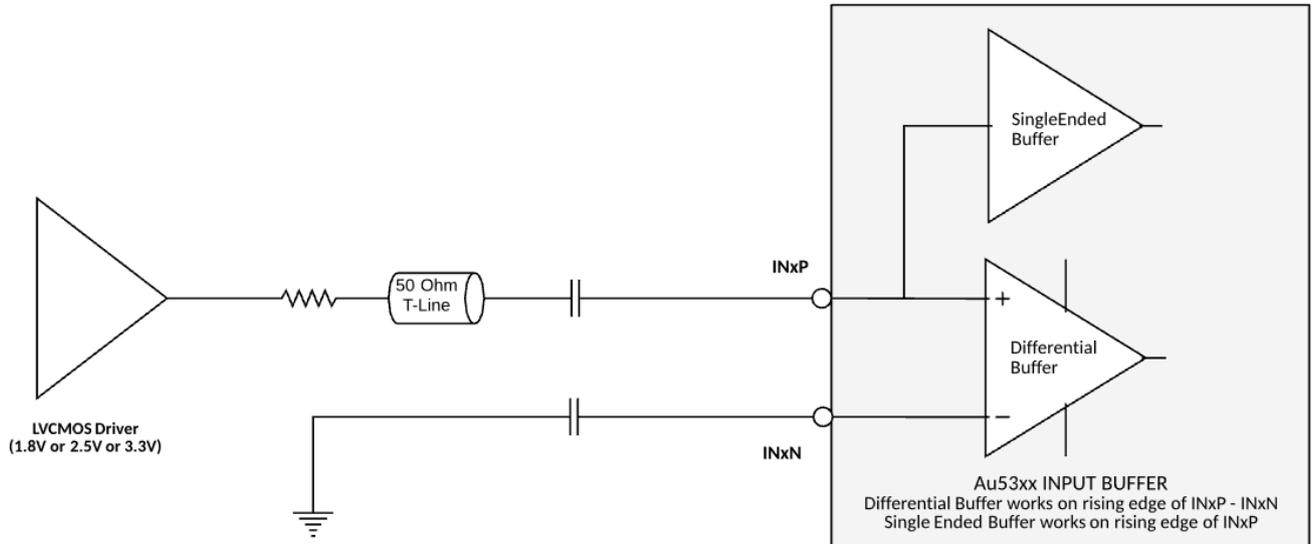
**Figure 39 AC Coupled Single Ended LVCMOS input without 50 Ohm Termination**
