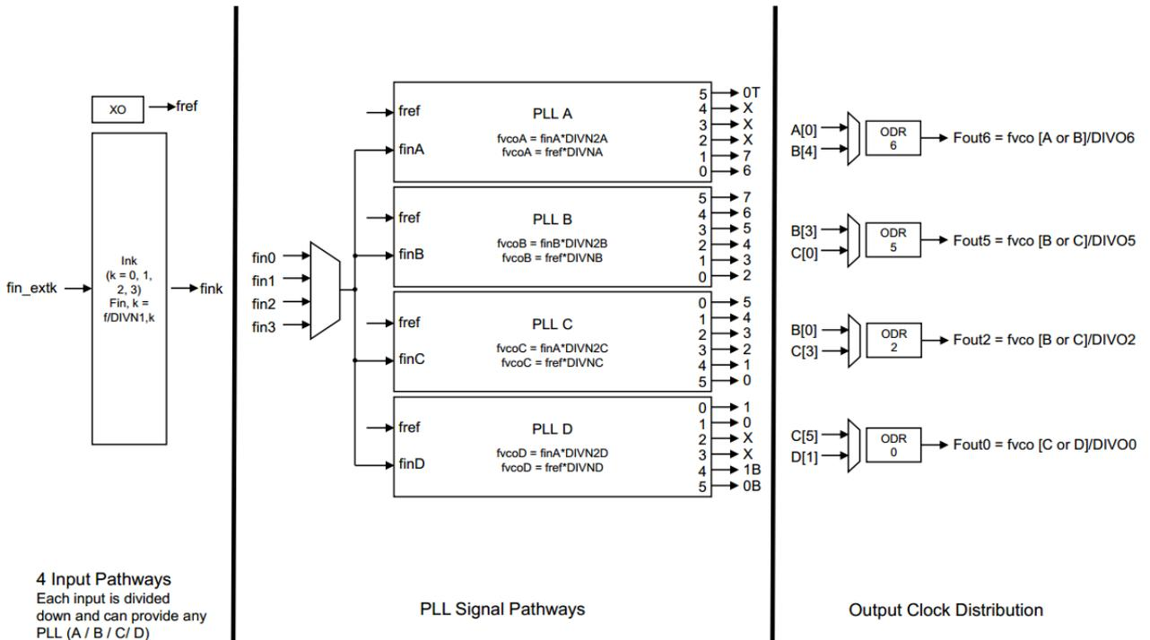
Figure 11 Au5314 & Au5324 Overall Hierarchy of Clocks
