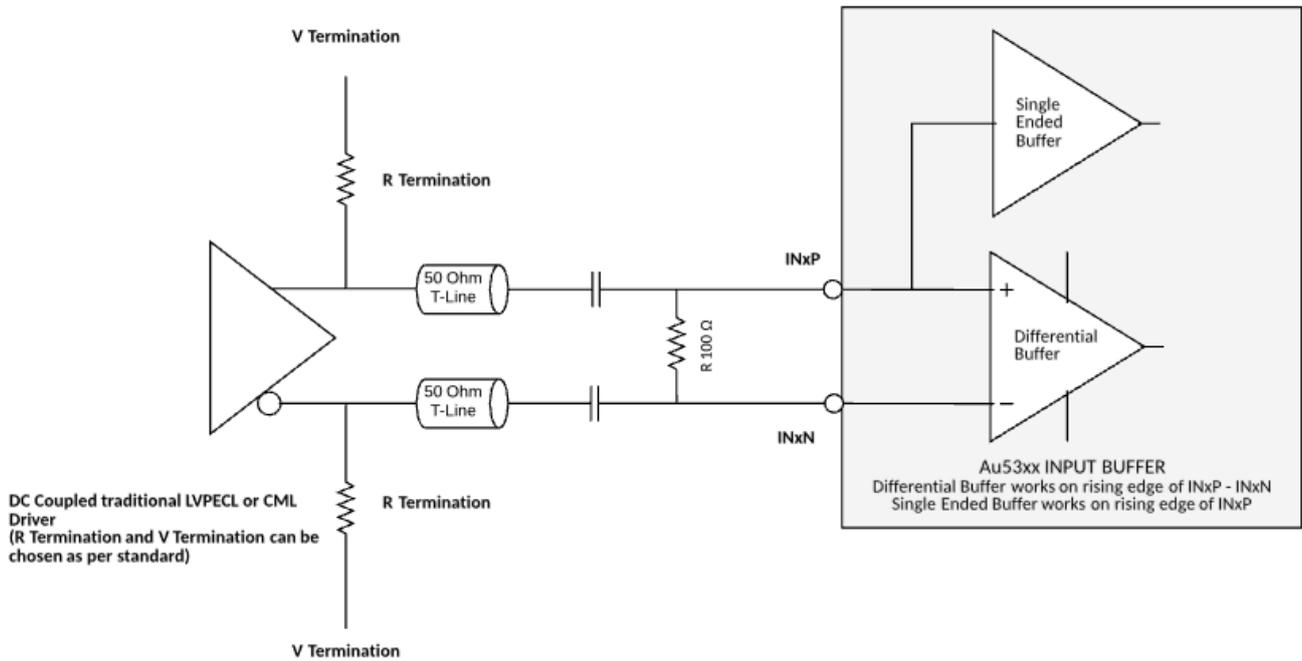
**Figure 36 AC Coupled Differential LVPECL or CML**
