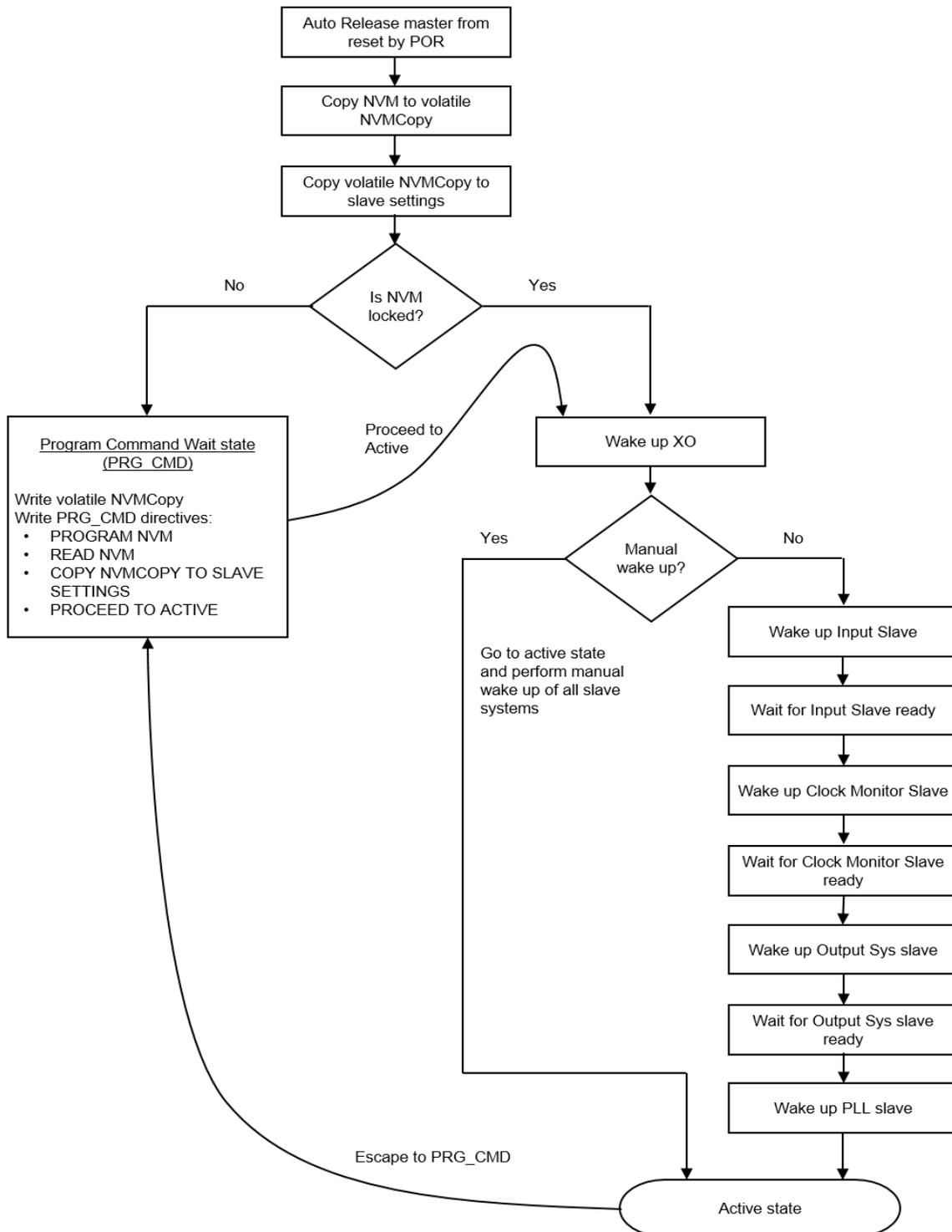
Figure 20 Master Wake-up Finite State Machine
