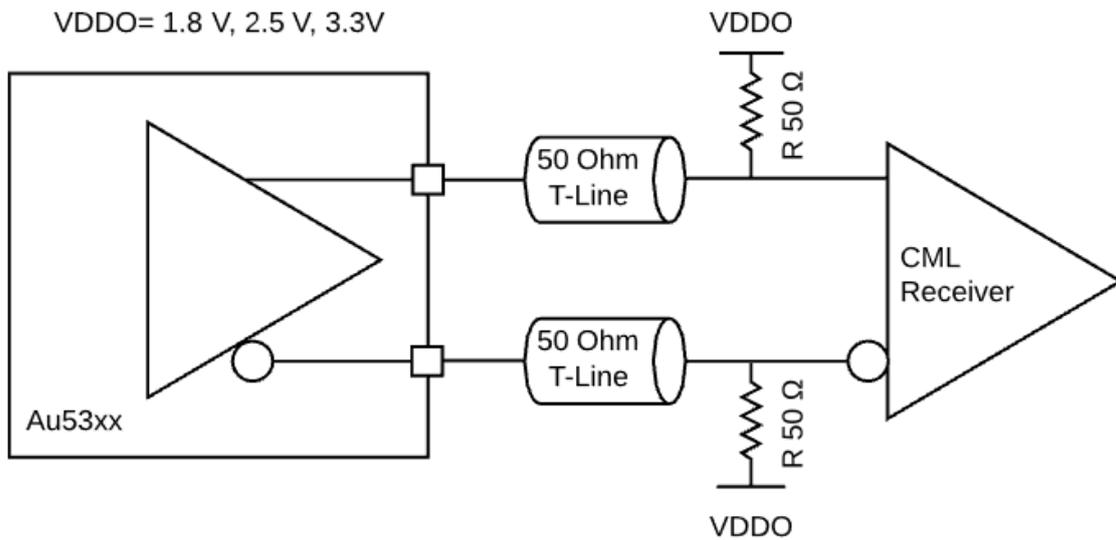
Traditional DC Coupled CML Receiver: **Use CML Standard for the Au53xx Output Driver**
