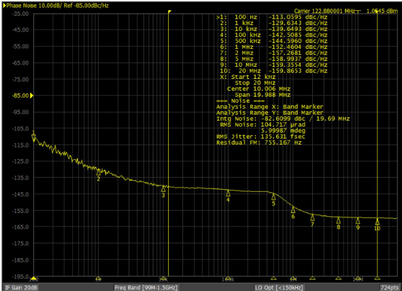
Figure 6 Representative Close In Phase Noise Measurement
