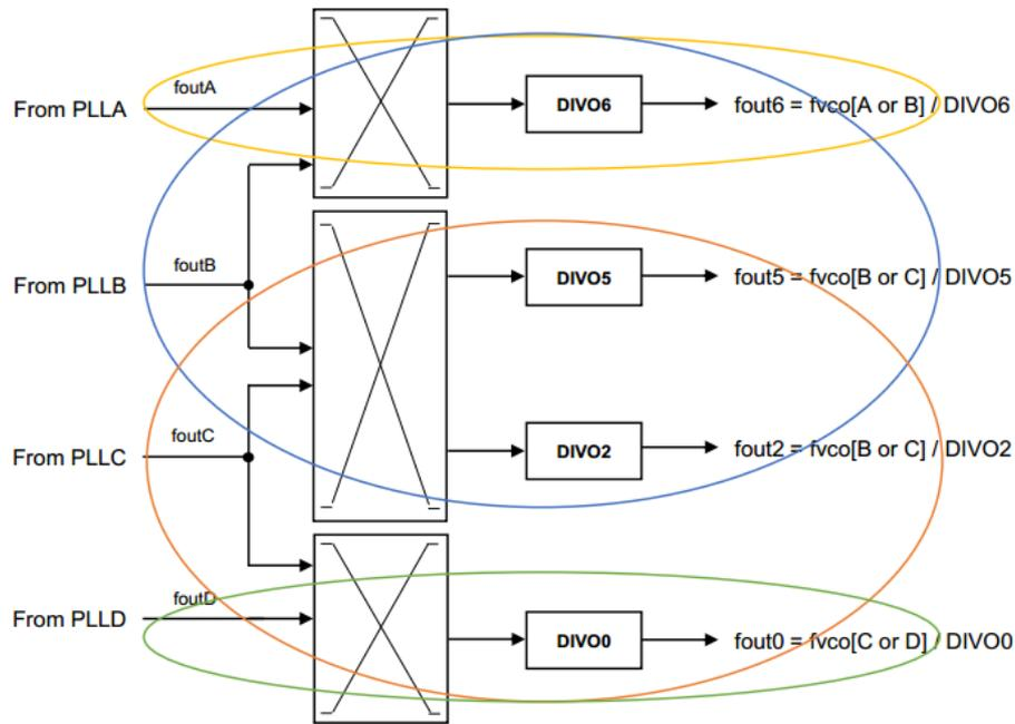
Figure 16 Au5314 & Au5324 Output Clock Distribution
