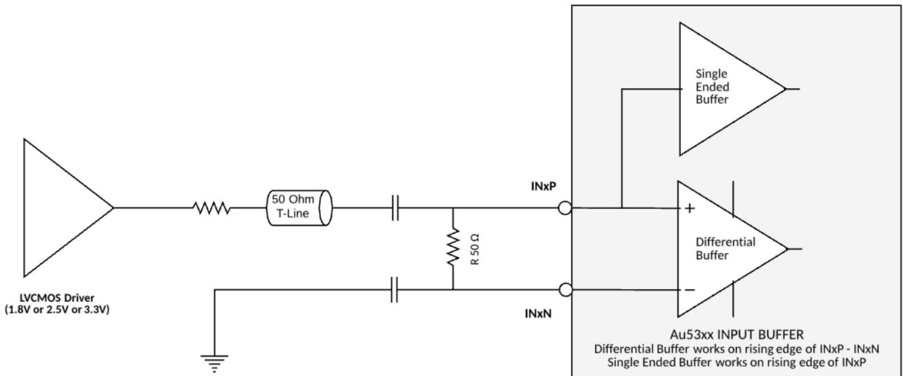
Figure 38 AC Coupled Single Ended Driver with 50 Ohm Termination on receiver (chip) side
