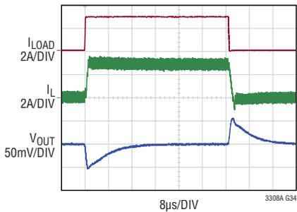
3.3V<sub>IN</sub> to 1.2V<sub>OUT</sub>, 2MHz Typical Application
