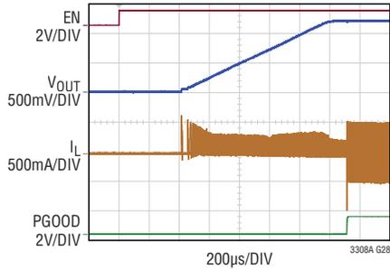
3.3V<sub>IN</sub> to 1.2V<sub>OUT</sub>, 2MHz Typical Application
