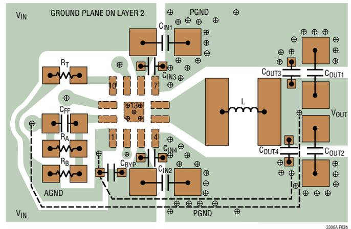
(b) With Capacitors  $C_{OUT1}$  and  $C_{OUT2}$  Rotated by  $90^\circ$ , Which Reduces High Frequency Output Ripple. Optional 0201 Capacitors  $C_{OUT3}$  and  $C_{OUT4}$  Further Improve the High Frequency Output Ripple. Five 5mil Vias Are Used within the EPAD. For Layouts Where 5mil Vias Are Not Allowed, It Is Recommended to Use Either Four 8mil Vias or a Single (Filled or Tented) 12mil Diameter Via.
