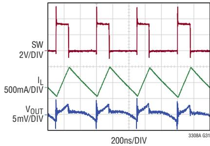
3.3V<sub>IN</sub> to 1.2V<sub>OUT</sub>, 2MHz Typical Application
