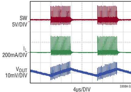
5.0V<sub>IN</sub> to 1.2V<sub>OUT</sub>, 2MHz Application
