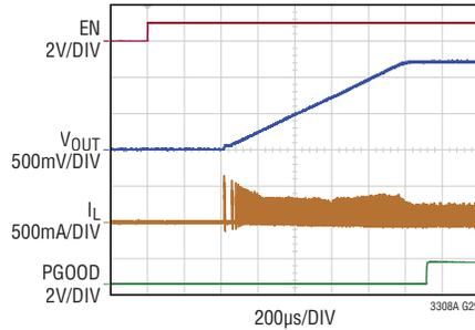
3.3V<sub>IN</sub> to 1.2V<sub>OUT</sub>, 2MHz Typical Application
