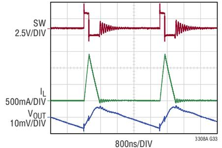
3.3V<sub>IN</sub> to 1.2V<sub>OUT</sub>, 2MHz Typical Application
