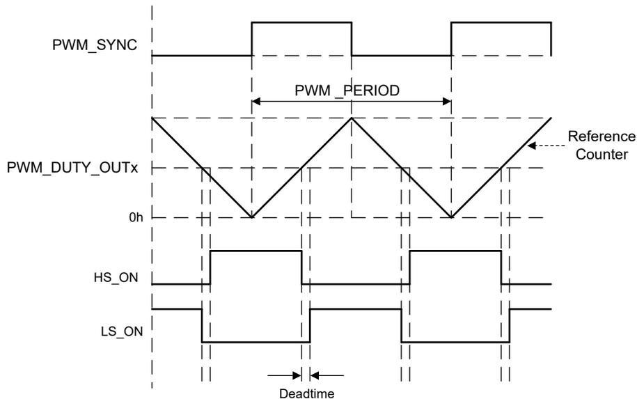
**Figure 8-11. PWM Synchronization in Up/down Mode (PWM\_OSC\_SYNC = 2h)**
