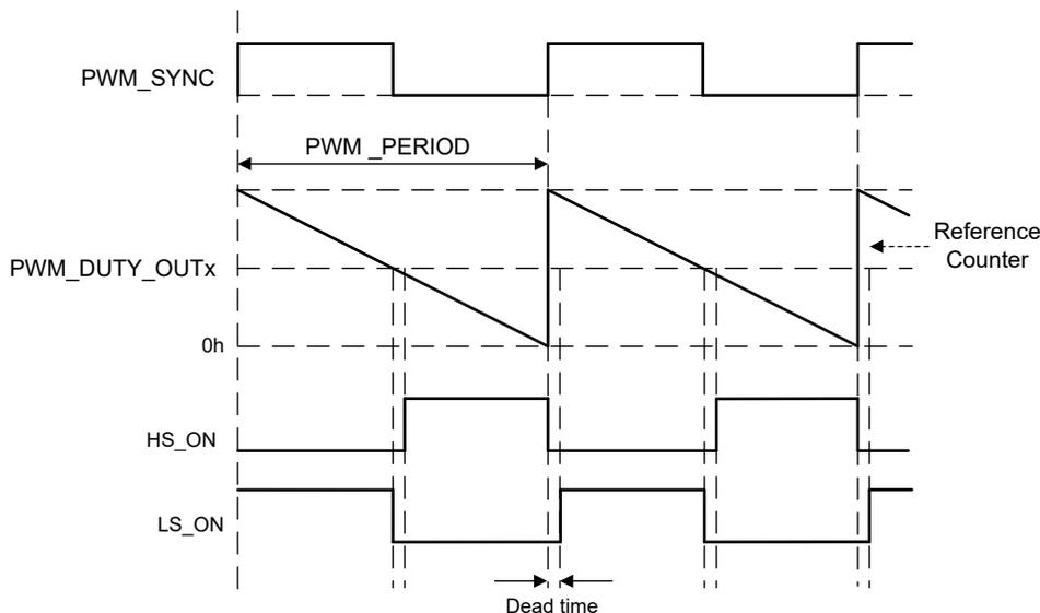
**Figure 8-13. PWM Synchronization in Down Mode (PWM\_OSC\_SYNC = 2h)**
