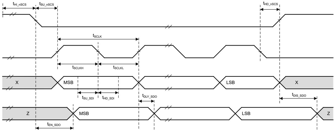
Figure 7-1. SPI Secondary Device Mode Timing Diagram
