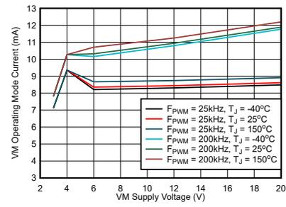
**Figure 7-3. Operating mode current over supply voltage**
