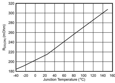
**Figure 7-2. R<sub>DS(ON)</sub> (high and low side combined) for MOSFETs over temperature, VM ≥ 6V**
