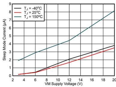
**Figure 7-4. Sleep current over supply voltage**
