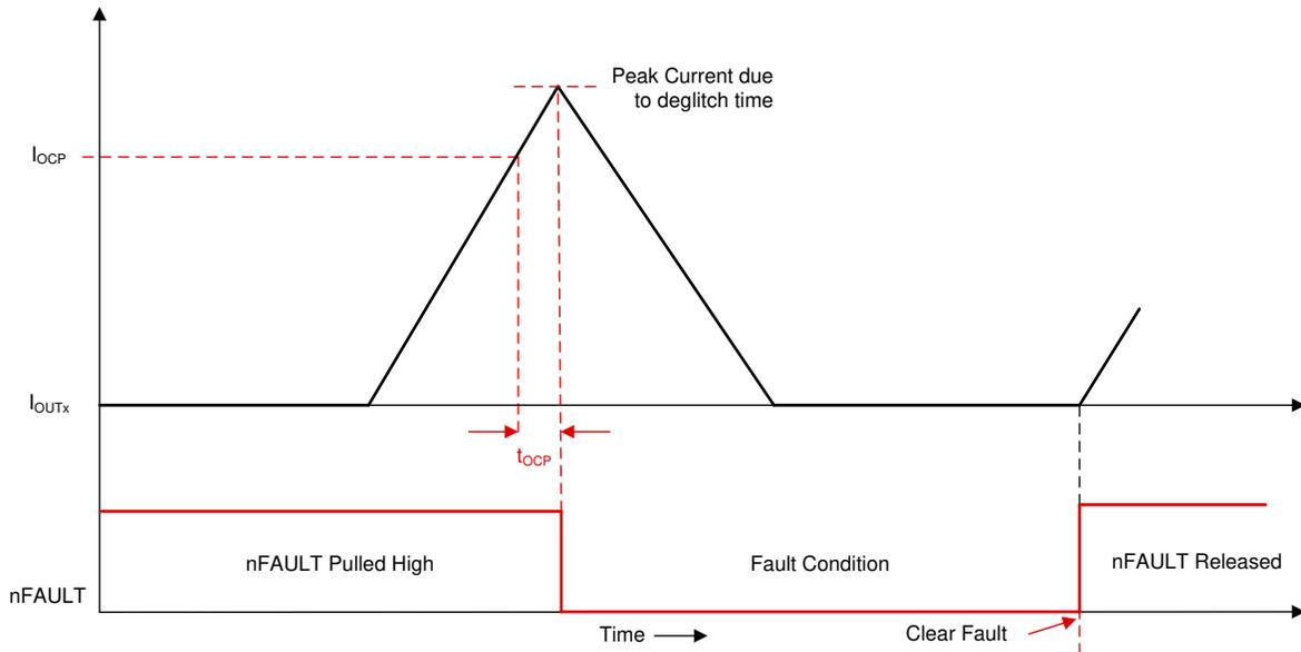
**Figure 8-32. Overcurrent Protection - Latched Shutdown Mode**
