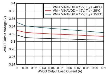
**Figure 7-5. AVDD regulator output voltage over load current**
