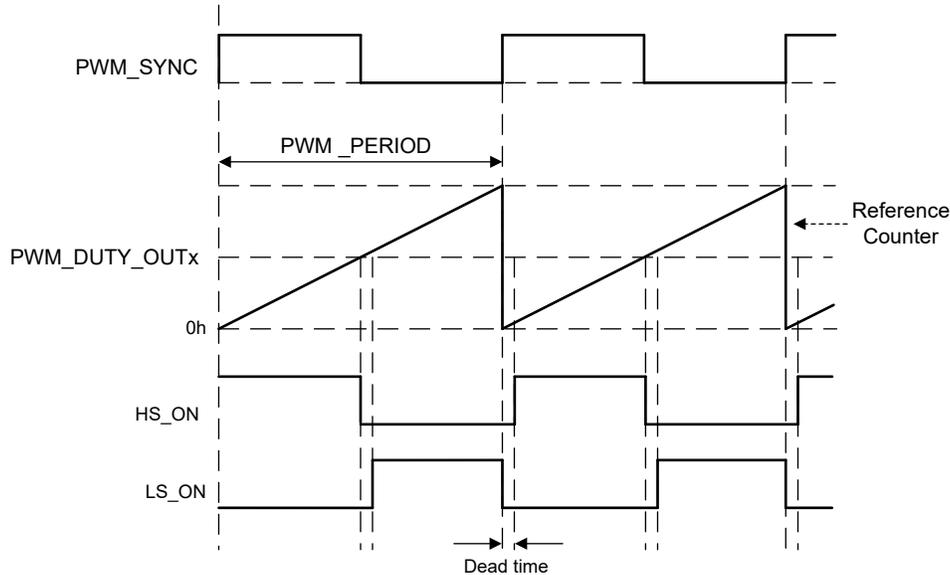
**Figure 8-12. PWM Synchronization in Up Mode (PWM\_OSC\_SYNC = 2h)**
