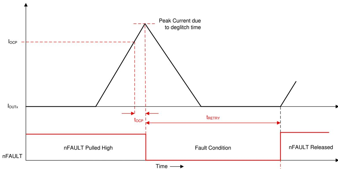
**Figure 8-33. Overcurrent Protection - Automatic Retry Mode**
