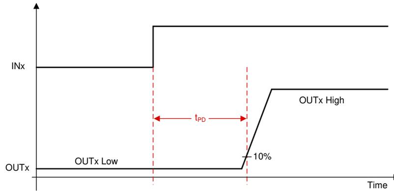
**Figure 8-22. Propagation Delay**
