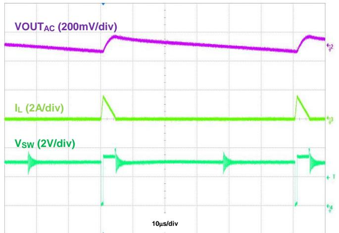
Figure 36. Output Voltage Ripple,  $V_{IN} = 3\text{V}$ ,  $V_{OUT} = 3.3\text{V}$ ,  $I_{OUT} = 50\text{mA}$
