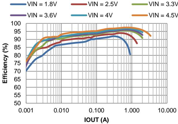
Figure 27. Efficiency vs. Output Current,  $V_{OUT} = 5.2\text{V}$
