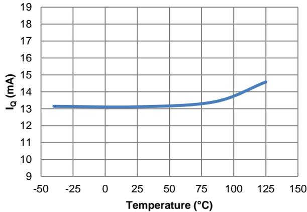
Figure 45.  $I_q$  vs. Temperature,
