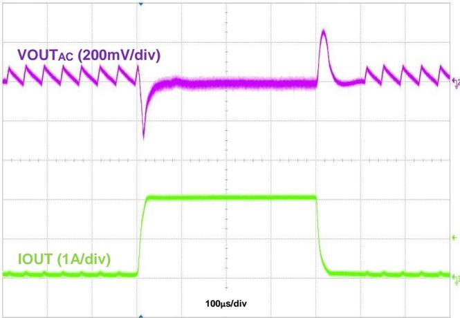
**Figure 40. Load Transient, IO<sub>UT</sub> = 50mA to 2A to 50mA**
