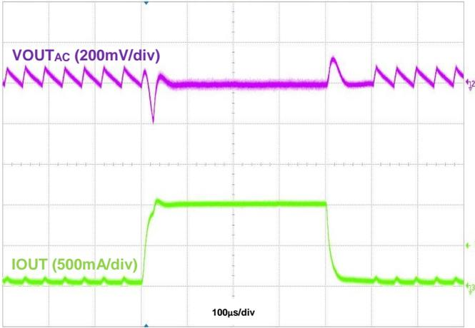
**Figure 38. Load Transient, IO<sub>UT</sub> = 50mA to 1A to 50mA**
