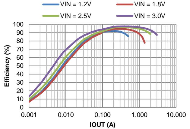
Figure 42. Efficiency vs. Output Current,  $V_{OUT} = 3.3\text{V}$
