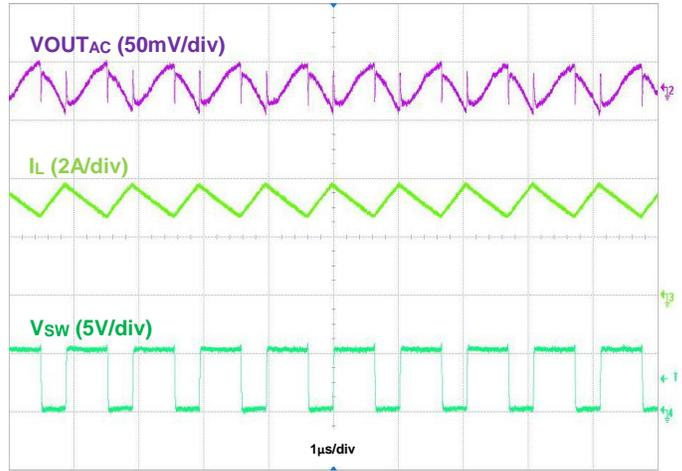
Figure 21. Output Voltage Ripple,  $V_{OUT} = 5.2\text{V}$ ,  $I_{OUT} = 2\text{A}$
