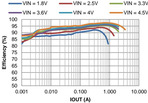
Figure 14. Efficiency vs. Output Current,  $V_{OUT} = 5.2\text{V}$
