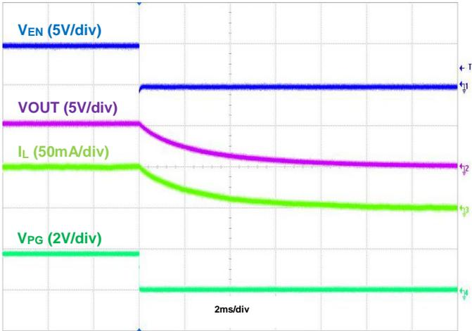
Figure 11. Shutdown Using EN,  $I_{OUT} = 50\text{mA}$
