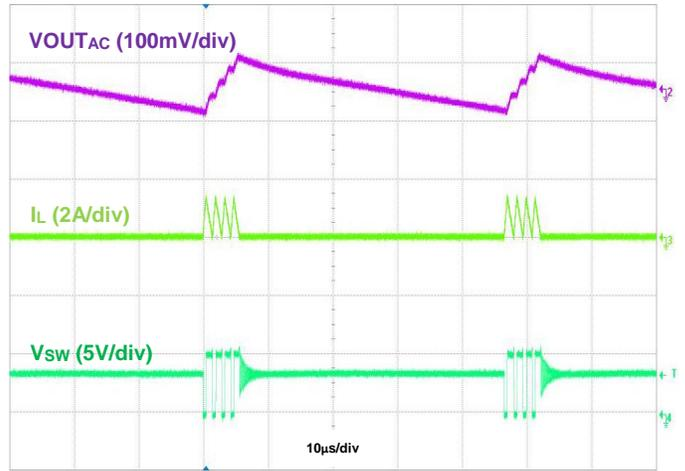
Figure 34. Output Voltage Ripple,  $V_{OUT} = 5.2\text{V}$ ,  $I_{OUT} = 50\text{mA}$
