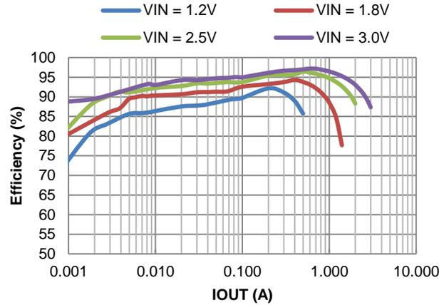
Figure 28. Efficiency vs. Output Current,  $V_{OUT} = 3.3\text{V}$
