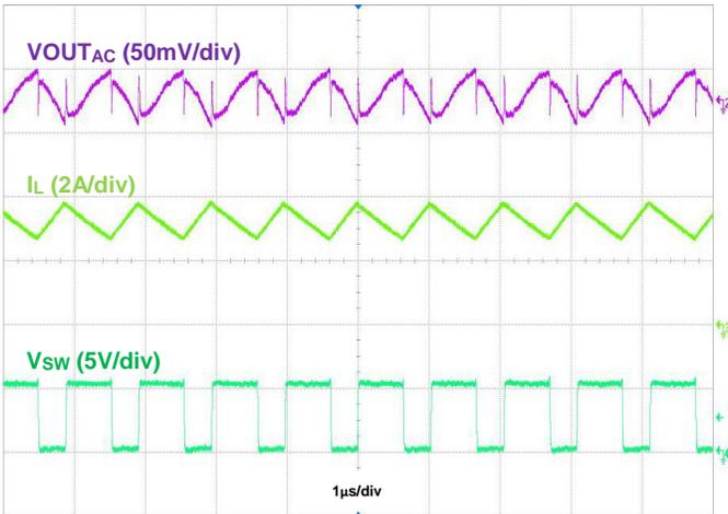
Figure 35. Output Voltage Ripple,  $V_{OUT} = 5.2\text{V}$ ,  $I_{OUT} = 2\text{A}$
