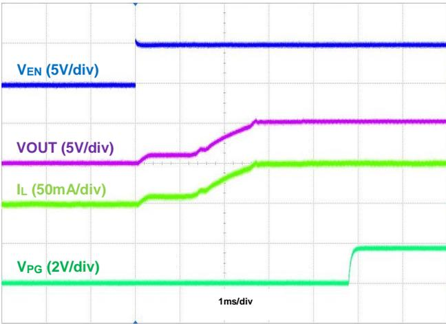
Figure 10. Startup Using EN,  $I_{OUT} = 50\text{mA}$
