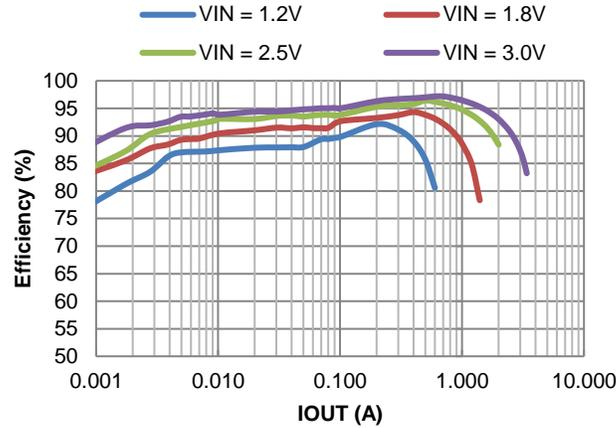
Figure 15. Efficiency vs. Output Current,  $V_{OUT} = 3.3\text{V}$
