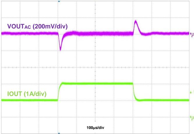
**Figure 39. Load Transient, IO<sub>UT</sub> = 1A to 2A to 1A**
