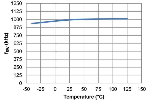
Figure 46.  $f_{sw}$  vs. Temperature,  $I_{OUT} = 0\text{A}$
