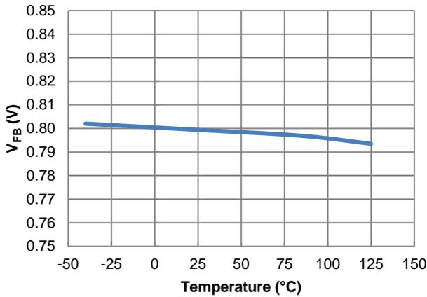
Figure 6. Feedback Voltage vs. Temperature,  $I_{OUT} = 1\text{A}$
