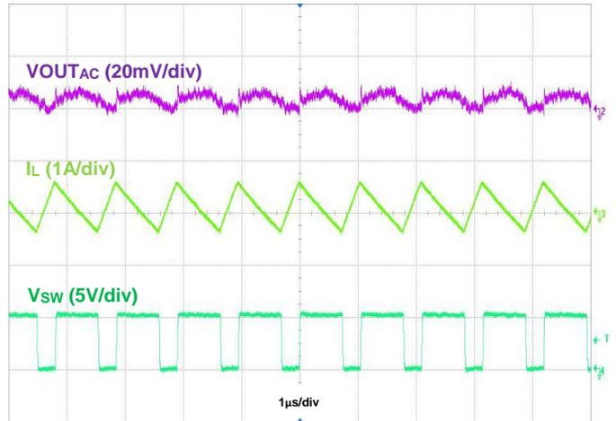
Figure 48. Output Voltage Ripple,  $V_{OUT} = 5.2\text{V}$ ,  $I_{OUT} = 50\text{mA}$
