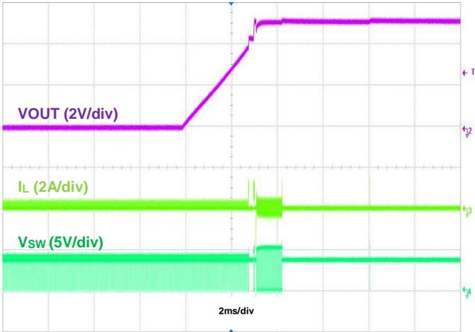
Figure 13. Output Short Recovery,  $I_{OUT} = 0\text{A}$
