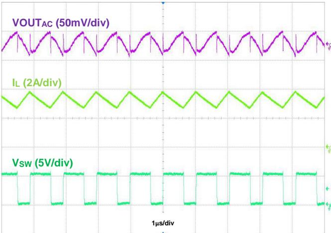
Figure 49. Output Voltage Ripple,  $V_{OUT} = 5.2\text{V}$ ,  $I_{OUT} = 2\text{A}$
