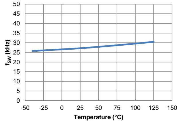
Figure 32.  $f_{sw}$  vs. Temperature,  $I_{OUT} = 0\text{A}$
