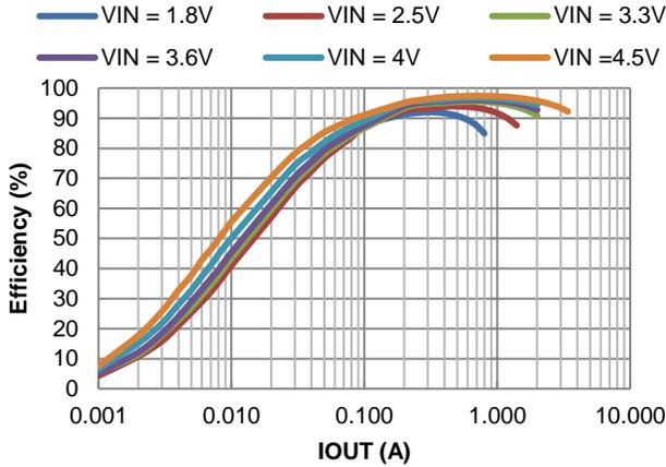
Figure 41. Efficiency vs. Output Current,  $V_{OUT} = 5.2\text{V}$
