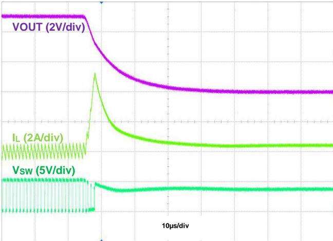
Figure 12. Output Short Protection,  $I_{OUT} = 0\text{A}$
