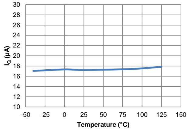
Figure 7.  $I_Q$  vs. Temperature,  $V_{EN} = V_{IN}$ ,  $V_{FB} = 1.0\text{V}$
