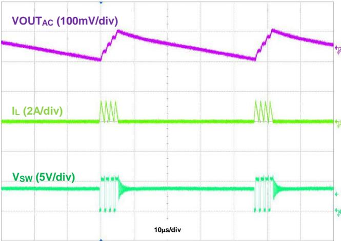
Figure 20. Output Voltage Ripple,  $V_{OUT} = 5.2\text{V}$ ,  $I_{OUT} = 50\text{mA}$
