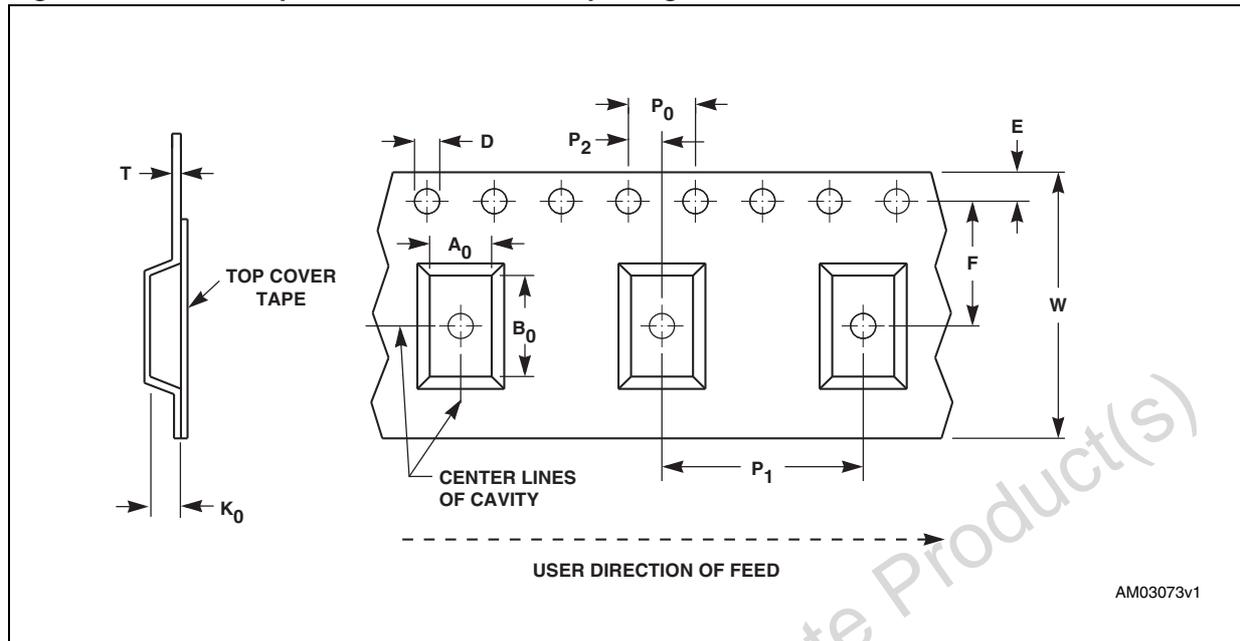
Table 30. Carrier tape dimensions for DFN8 and TDFN8 packages
