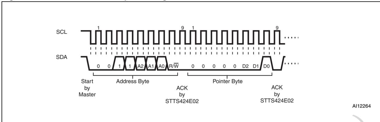
Figure 5. SMBus/I<sup>2</sup>C write to pointer register, followed by a read data word
