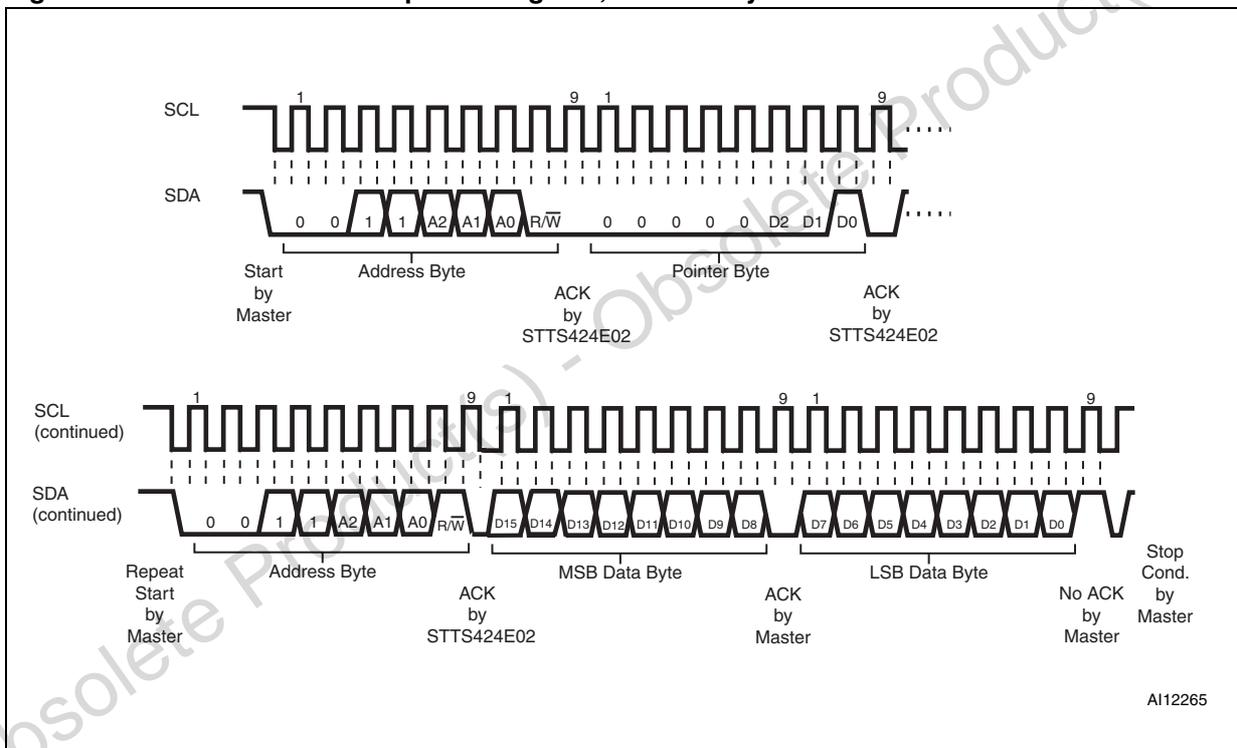
Figure 6. SMBus/I<sup>2</sup>C write to pointer register, followed by a write data word
