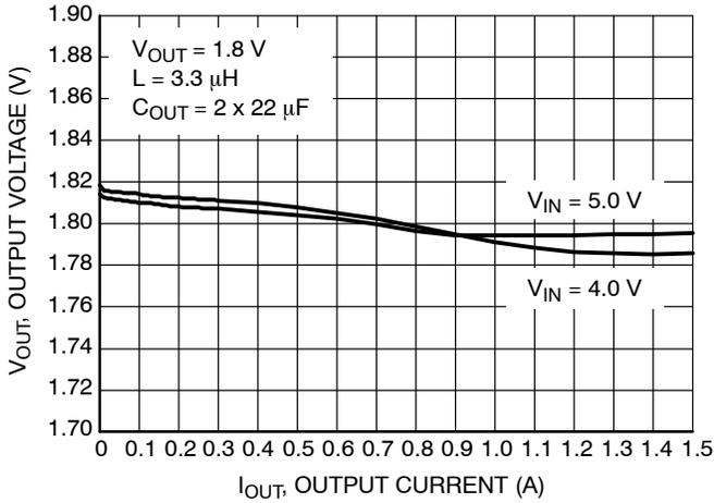
Figure 11. Load Regulation for  $V_{OUT} = 1.8\text{ V}$
