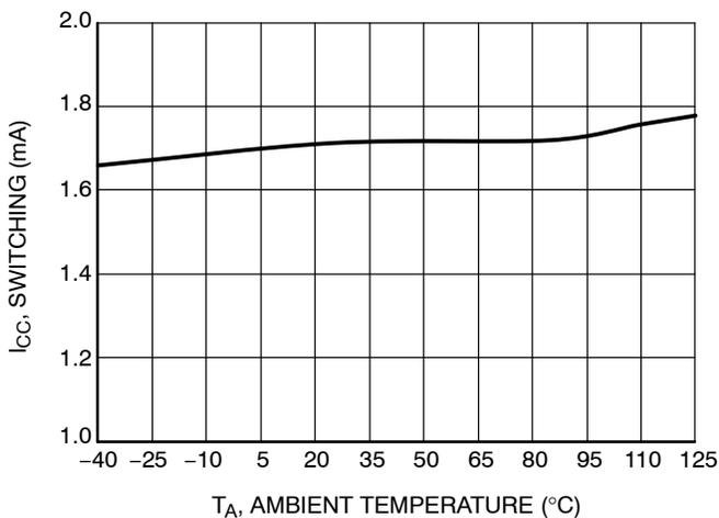
**Figure 7. Quiescent Current Into  $V_{CC}$  vs. Temperature**
