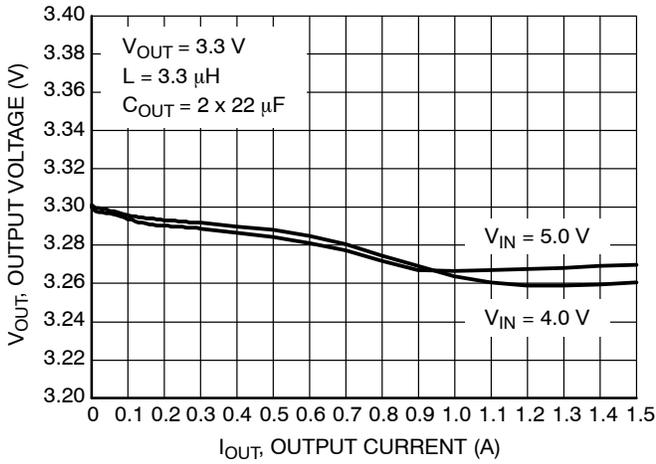
Figure 9. Load Regulation for  $V_{OUT} = 3.3\text{ V}$
