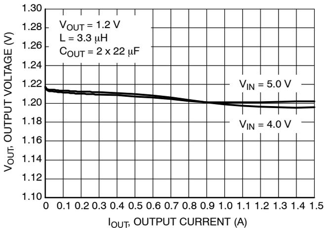
Figure 13. Load Regulation for  $V_{OUT} = 1.2\text{ V}$
