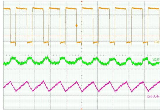
( $V_{IN} = 5\text{ V}$ ,  $I_{LOAD} = 700\text{ mA}$ ,  $L = 3.3\text{ }\mu\text{H}$ ,  $C_{OUT} = 2 \times 22\text{ }\mu\text{F}$ )
