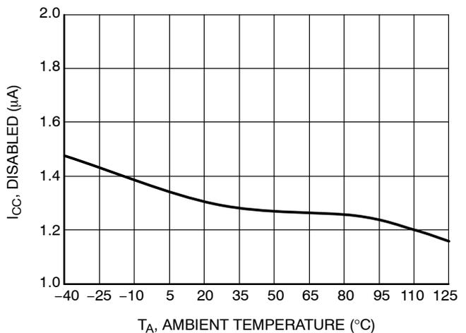
**Figure 8. Quiescent Current Into  $V_{CC}$  vs. Temperature**
