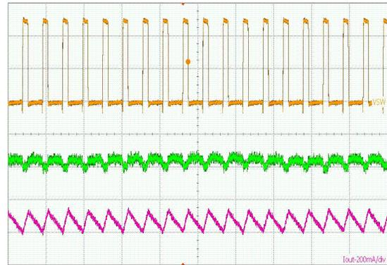
( $V_{IN} = 5\text{ V}$ ,  $I_{LOAD} = 400\text{ mA}$ ,  $L = 3.3\text{ }\mu\text{H}$ ,  $C_{OUT} = 2 \times 22\text{ }\mu\text{F}$ )
