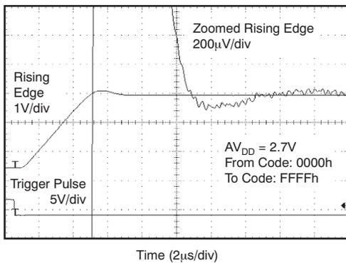
**Figure 106. Full-Scale Settling Time: 2.7-V Rising Edge**
