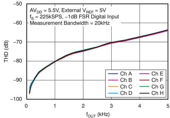
Figure 50. Third Harmonic Distortion vs Output Frequency
