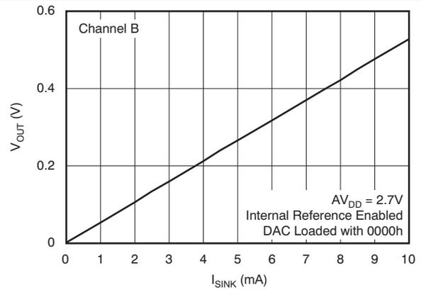
**Figure 97. Sink Current at Negative Rail (All Grades)**
