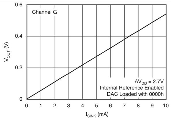
**Figure 99. Sink Current at Negative Rail (All Grades)**
