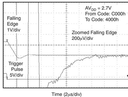
**Figure 109. Half-Scale Settling Time: 2.7-V Falling Edge**
