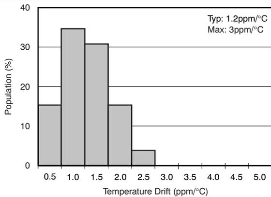
**Figure 6. Reference Output Temperature Drift (0°C to +125°C, Grades C and D)**
