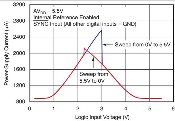
**Figure 44. Power-Supply Current vs Logic Input Voltage**
