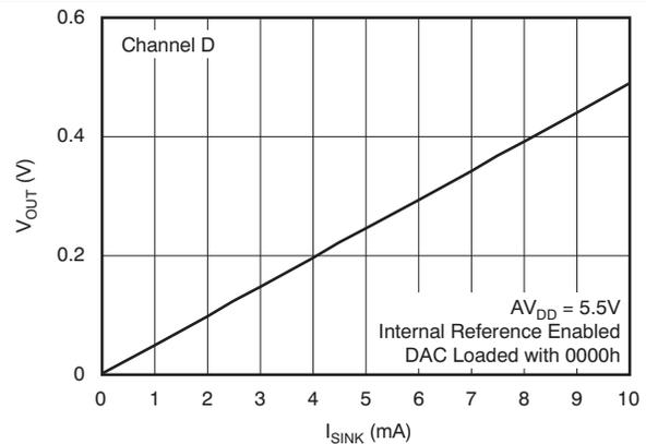
**Figure 35. Sink Current at Negative Rail (All Grades)**
