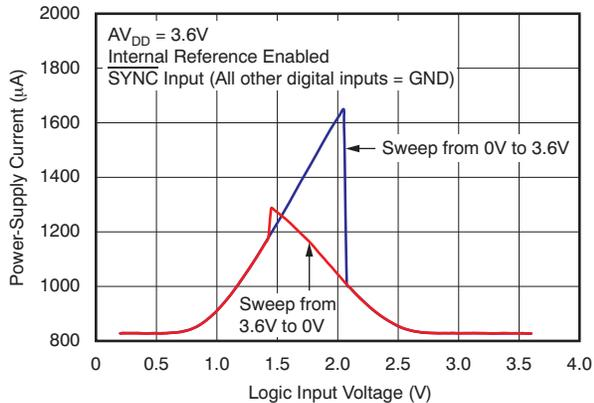
Figure 72. Power-Supply Current vs Logic Input Voltage
