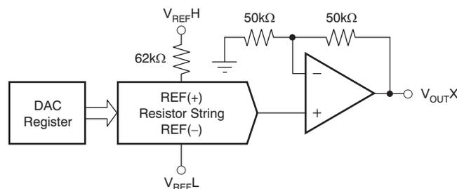
Figure 120. Device Architecture
