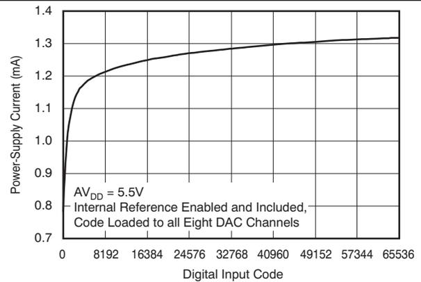
Figure 39. Power-Supply Current vs Digital Input Code
