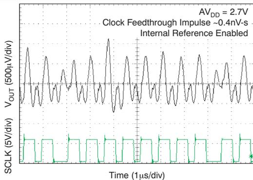
**Figure 110. Clock Feedthrough 2.7 V, 2 Mhz, Midscale**
