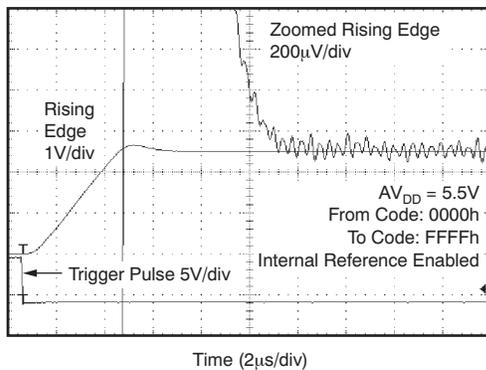
Figure 52. Full-Scale Settling Time: 5-V Rising Edge
