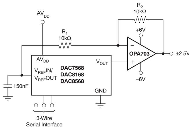
Figure 129. Bipolar Output Range Using Internal Reference
