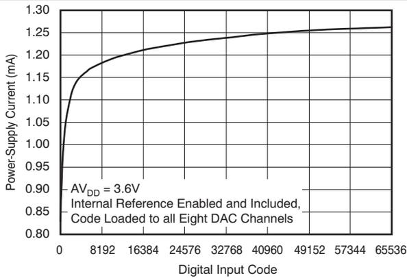
Figure 68. Power-Supply Current vs Digital Input Code
