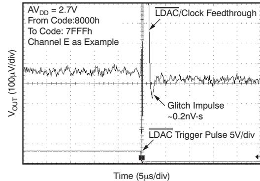
Figure 115. Glitch Energy: 2.7 V, 1-LSB Step, Falling Edge
