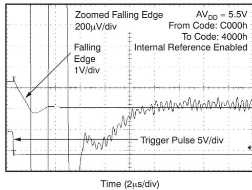
**Figure 55. Half-Scale Settling Time: 5-V Falling Edge**
