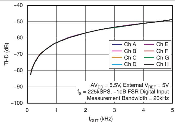
Figure 49. Second Harmonic Distortion vs Output Frequency
