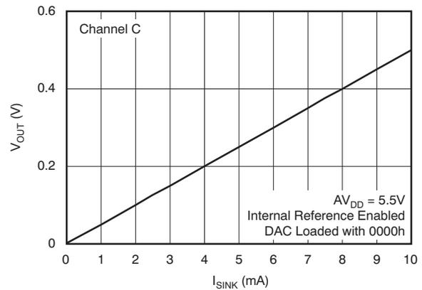
**Figure 33. Sink Current at Negative Rail (All Grades)**
