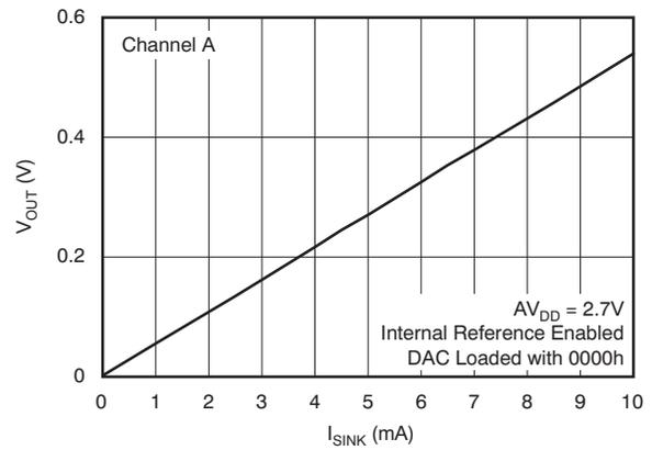
**Figure 95. Sink Current at Negative Rail (All Grades)**
