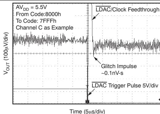
Figure 61. Glitch Energy: 5 V, 1-LSB Step, Falling Edge
