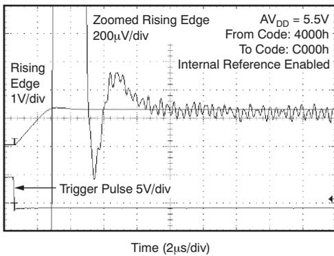
**Figure 54. Half-Scale Settling Time: 5-V Rising Edge**
