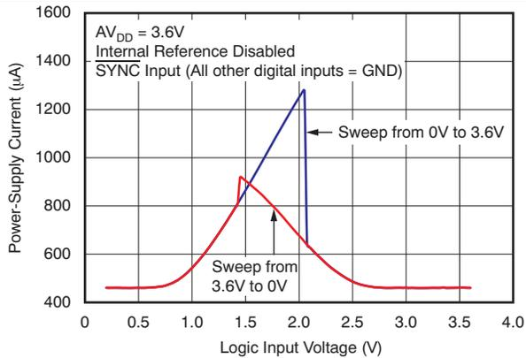
Figure 70. Power-Supply Current vs Logic Input Voltage
