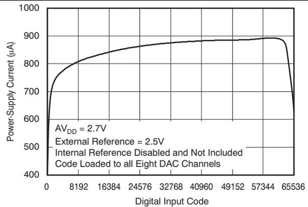
Figure 101. Power-Supply Current vs Digital Input Code
