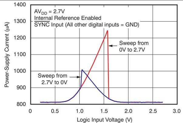
Figure 103. Power-Supply Current vs Logic Input Voltage
