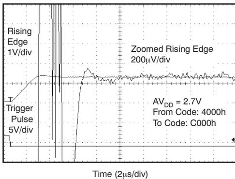
**Figure 108. Half-Scale Settling Time: 2.7-V Rising Edge**
