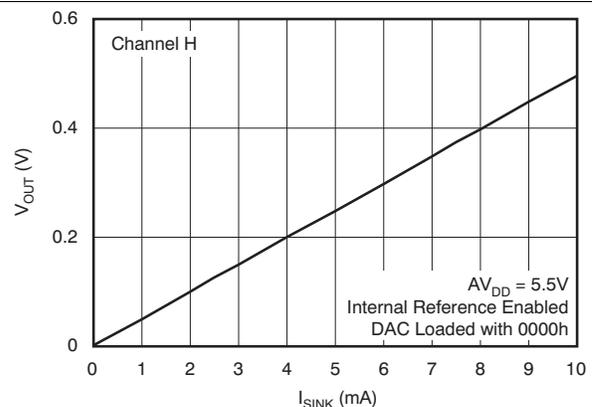
**Figure 37. Sink Current at Negative Rail (All Grades)**
