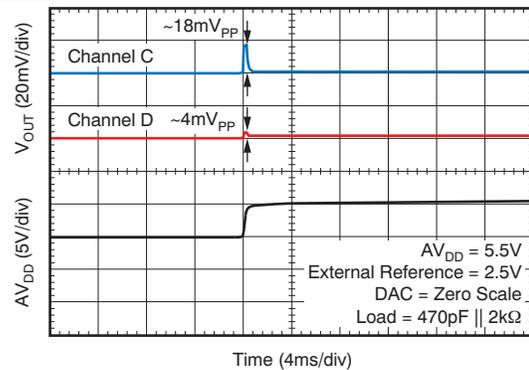
**Figure 57. Power-On Glitch Reset to Zero Scale**
