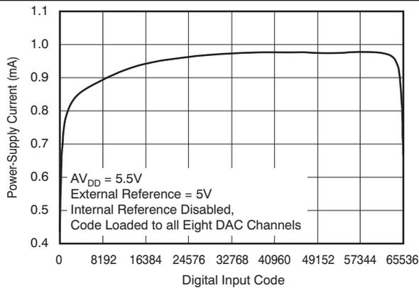
Figure 38. Power-Supply Current vs Digital Input Code
