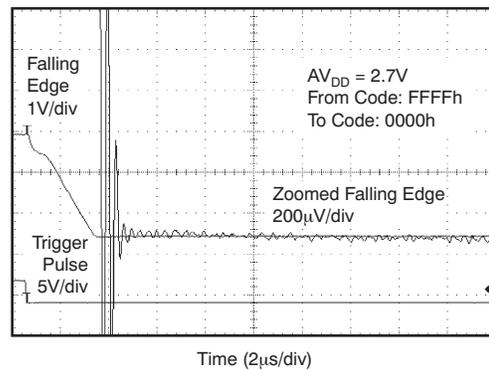
**Figure 107. Full-Scale Settling Time: 2.7-V Falling Edge**
