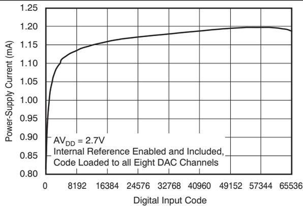
Figure 100. Power-Supply Current Vs Digital Input Code
