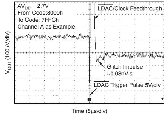
Figure 117. Glitch Energy: 2.7 V, 4-LSB Step, Falling Edge
