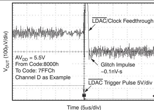
Figure 63. Glitch Energy: 5 V, 4-LSB Step, Falling Edge
