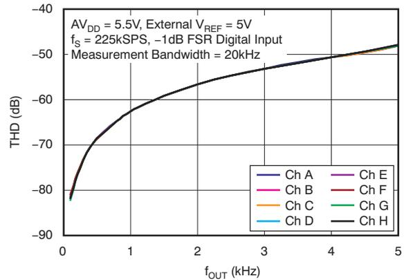
Figure 51. Total Harmonic Distortion vs Output Frequency
