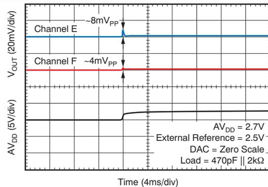
**Figure 111. Power-On Glitch Reset to Zero Scale**
