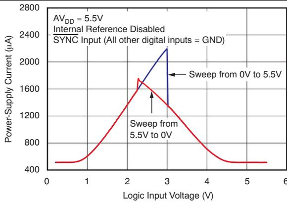
**Figure 43. Power-Supply Current vs Logic Input Voltage**
