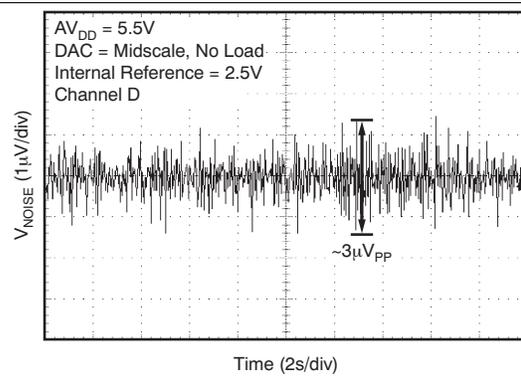
**Figure 67. DAC Output Noise 0.1 Hz to 10 Hz**
