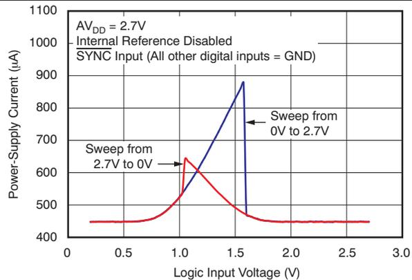
Figure 102. Power-Supply Current vs Logic Input Voltage
