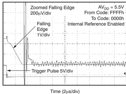
Figure 53. Full-Scale Settling Time: 5-V Falling Edge
