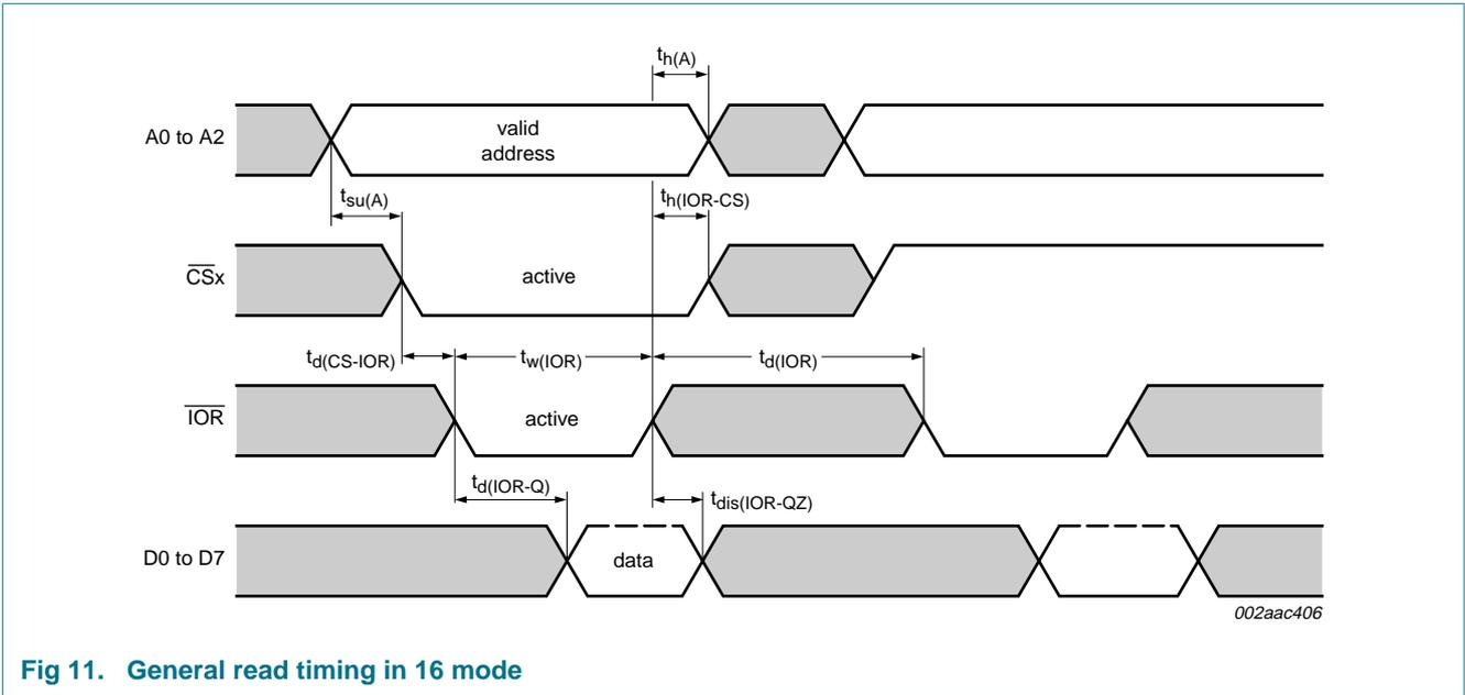
Fig 11. General read timing in 16 mode
