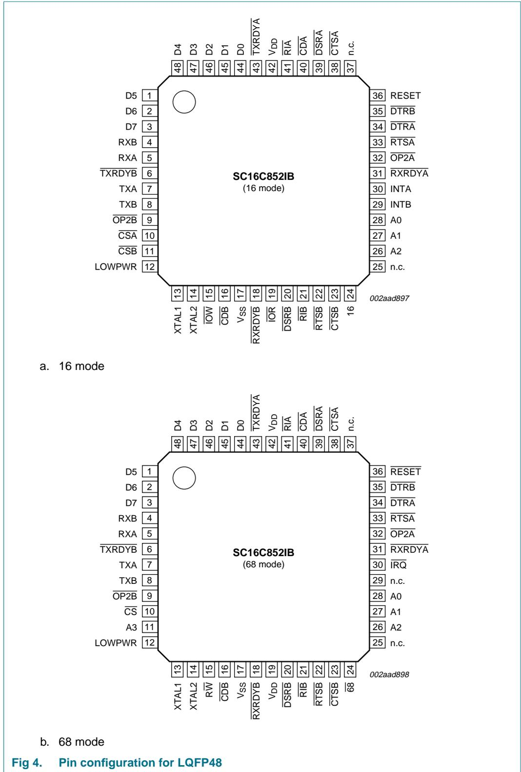
Fig 4. Pin configuration for LQFP48
