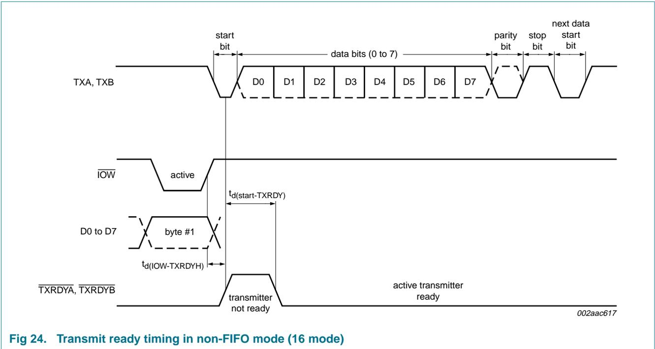
Fig 24. Transmit ready timing in non-FIFO mode (16 mode)
