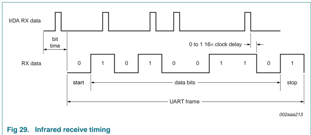
Fig 29. Infrared receive timing
