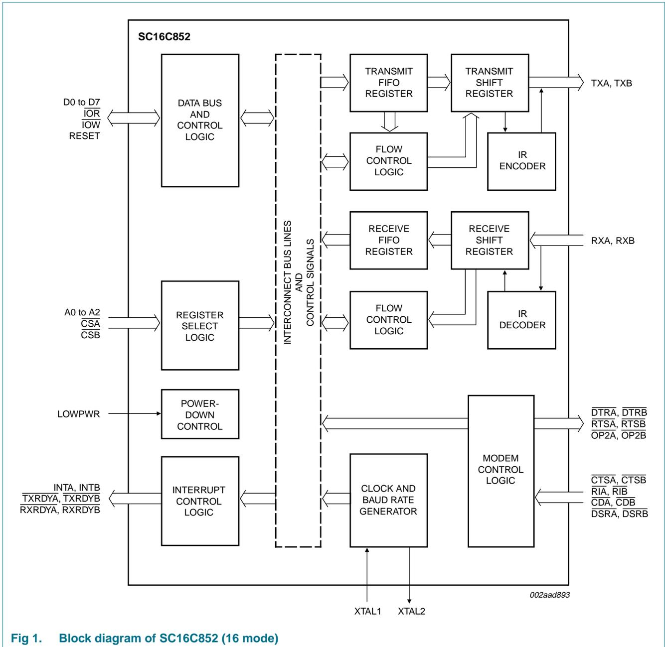
Fig 1. Block diagram of SC16C852 (16 mode)
