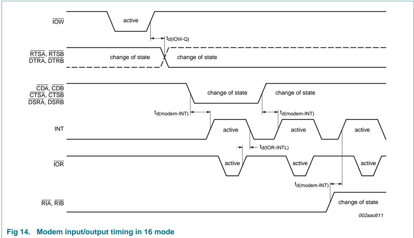
Fig 14. Modem input/output timing in 16 mode
