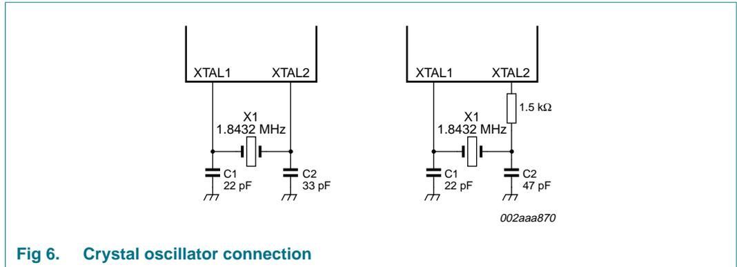
Fig 6. Crystal oscillator connection
