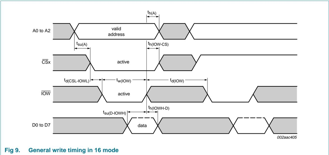
Fig 9. General write timing in 16 mode
