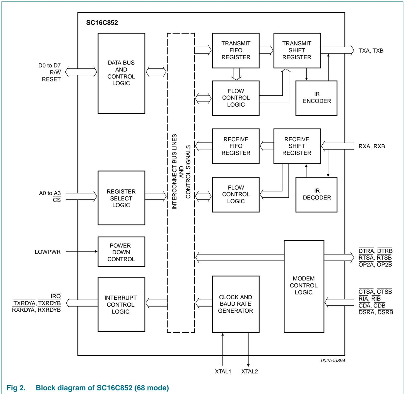
Fig 2. Block diagram of SC16C852 (68 mode)
