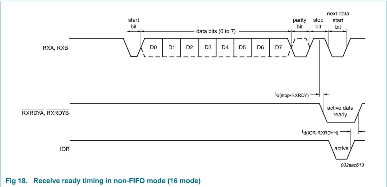
Fig 18. Receive ready timing in non-FIFO mode (16 mode)
