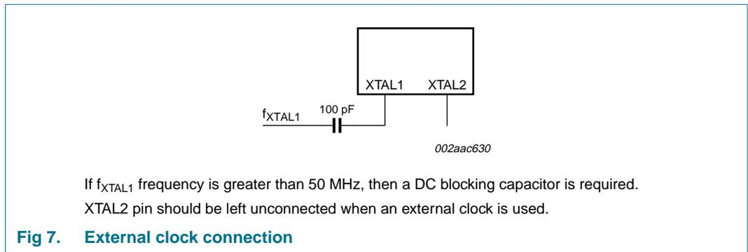
Fig 7. External clock connection
