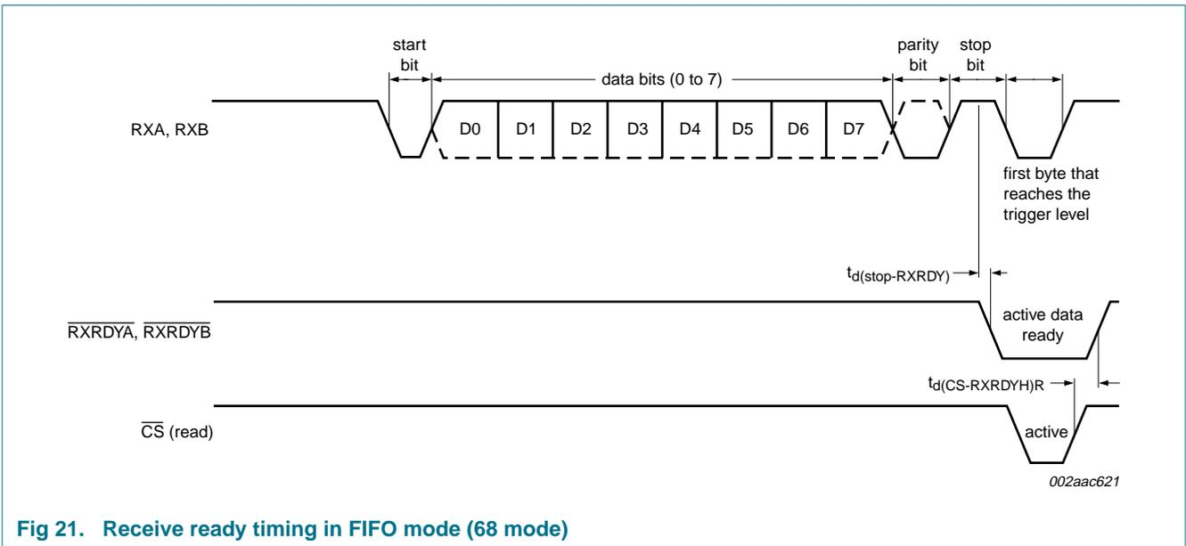
Fig 21. Receive ready timing in FIFO mode (68 mode)
