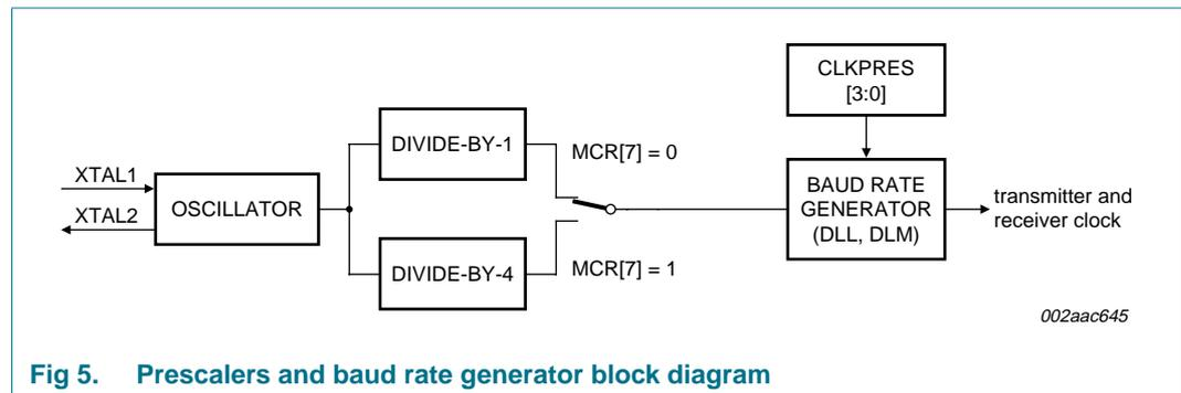
Fig 5. Prescalers and baud rate generator block diagram
