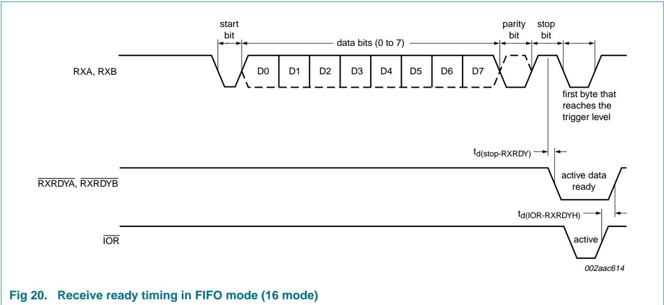
Fig 20. Receive ready timing in FIFO mode (16 mode)
