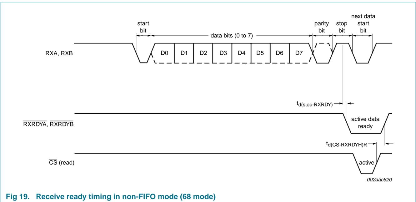
Fig 19. Receive ready timing in non-FIFO mode (68 mode)
