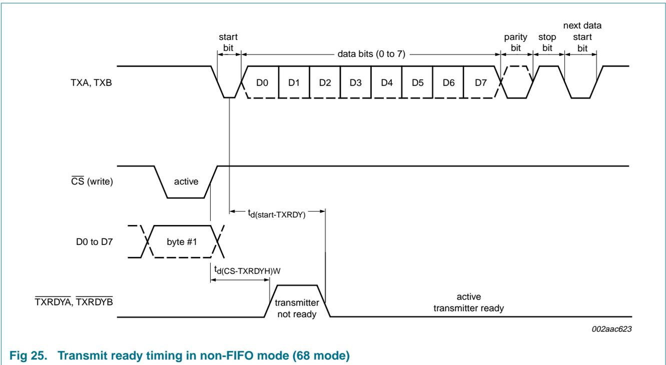
Fig 25. Transmit ready timing in non-FIFO mode (68 mode)
