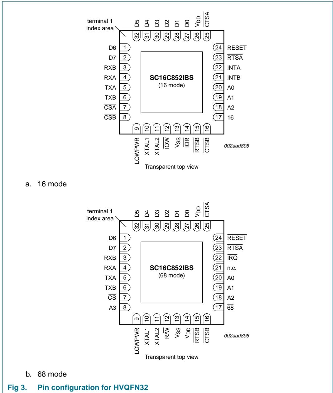
Fig 3. Pin configuration for HVQFN32
