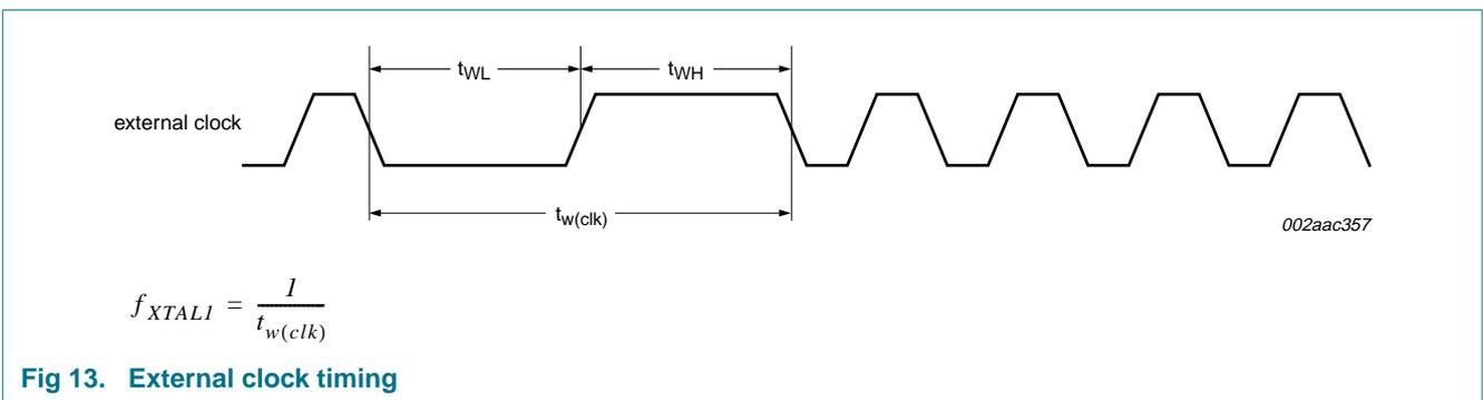
Fig 13. External clock timing
